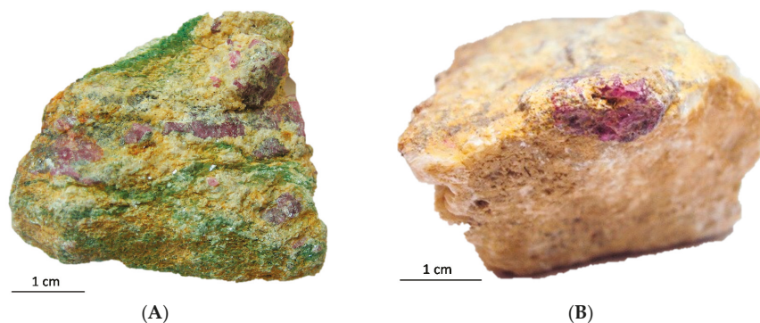
Figure 4. Images of hand specimens of Snezhnoe ruby-bearing rocks with: (A) ruby + plagioclase (albite–andesine) + muscovite (variety fuchsite) mineral paragenesis; (B) ruby + calcite mineral paragenesis. The images were modified from [11].
