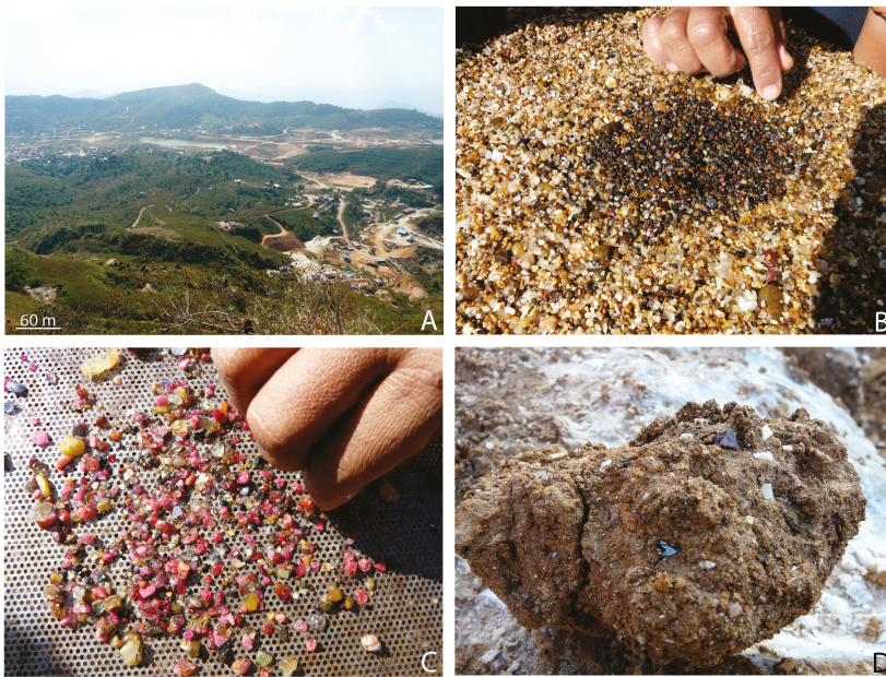
Figure 56. Different aspects of the gem placers in the Mogok Stone Track, Myanmar (in January 2015). (A) Panoramic view of the primary deposits mined in marble on the flank of the hills (foreground view) and secondary deposits, i.e., placers, mined in the valley (background); (B) image of the gem-bearing material called ‘byon’ enriched in gravels and sand. The concentration of heavy minerals is visible and is composed of iron oxides, corundum, quartz, and pieces of marble; (C) concentration of gem minerals (ruby, spinel, and sapphire) in the pan of a miner; and (D) sedimentary breccia formed in a cave placer karst. The breccia formed from an argillite containing crystals of spinel, plates of graphite, and fragments of marble and quartz. Size of the breccia sample around 15 cm long. Photo: Gaston Giuliani.
