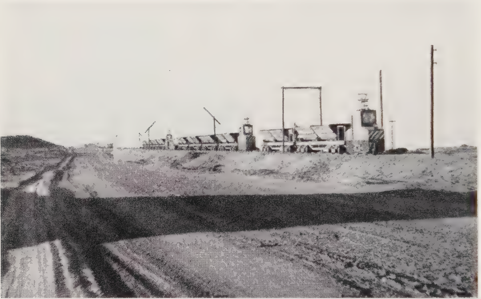
Fig. 12—Main haulage. Ten-ton electric locomotive with 5 cu. metre trucks
