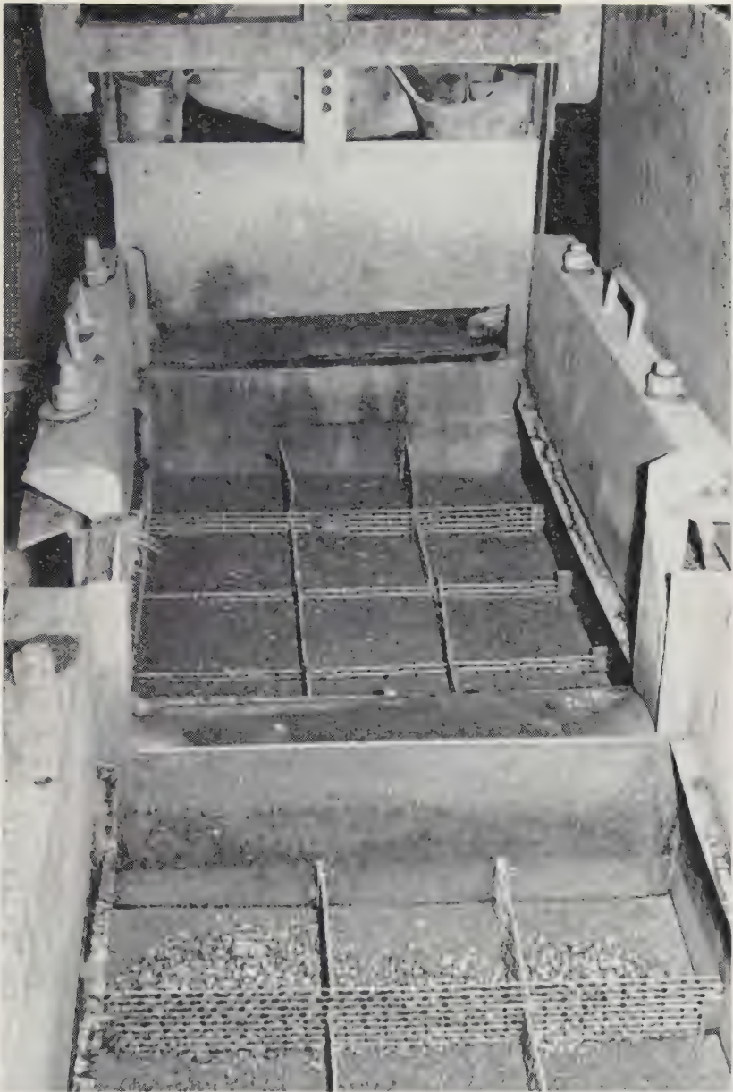
Fig. 1 Photograph showing divisions in jig screen compartments and feed distribution plate, as viewed from the tailings end
