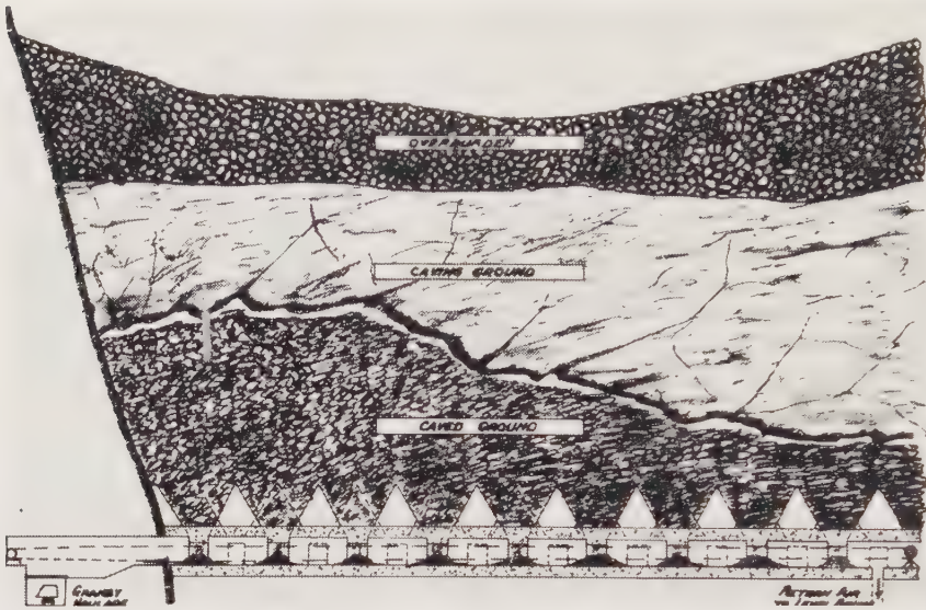
Fig. 4—Section along scraper drift
