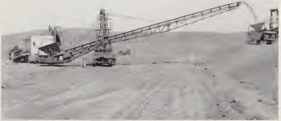
Fig. 8—Mobile stacker conveyor mounted on Sherman tank hull
