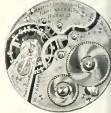
No. 978 Open Face. Nickel, 4 Plate Movement, 17 Extra Fine Jewels in Settings, Double Roller Escapement, Sapphire Pallets, Steel Escape Wheel, Micrometric Regulator, Breguet Hairspring, Compensation Balance, Double Sunk Dial, Adjusted to Temperature, Isochronism and Five Positions, $23.00
