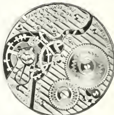
N.W. No. 993 Hunting. No. 992 Open Face. Nickel, 4 Plate Movement, 21 Extra Fine Ruby Jewels in Gold Settings, Double Roller Escapement, Sapphire Pallets, Gold Center Wheel, Steel Escape Wheel, Micrometric Regulator, Breguet Hairspring, Double Sunk Dial, Compensation Balance, Breguet Hairspring, Adjusted to Temperature, Isochronism and Five Positions, $38.00
