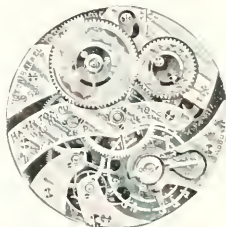
No. 952 Open Face. Nickel, Bridge Movement, Pendant or Lever Set, 19 Extra Fine Ruby Jewels in Gold Settings, Patent Motor Barrel, Steel Escape Wheel, Double Roller Escapement, Sapphire Pallets, Micrometric Regulator, Breguet Hairspring, Compensation Balance, Double Sunk Dial, Adjusted to Temperature, Isochronism and Five Positions, $47.50
