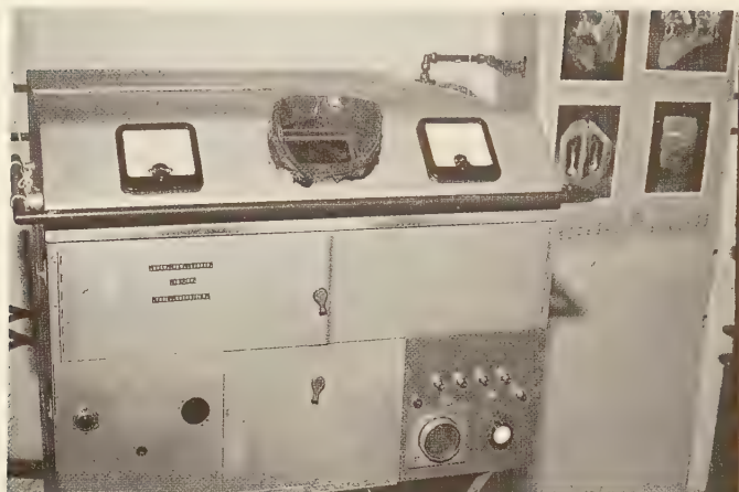
Figure 7.6 Viewing chamber of X-ray set (Photo: A Jobbins)
