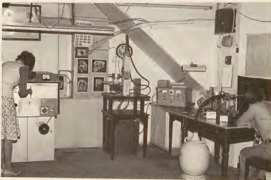
Figure 7.7 General scene in pearl-testing laboratory; centre, X-ray powder diffraction camera; left, checking X-ray fluorescence; right, freezing diamonds to enhance their spectra (Photo: A Jobbins)
