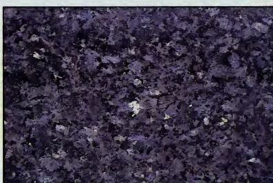
6 Norite, or "Blue Granite," is made principally of bluish feldspars. It is widely used for building facades, including the Chrysler Building.
