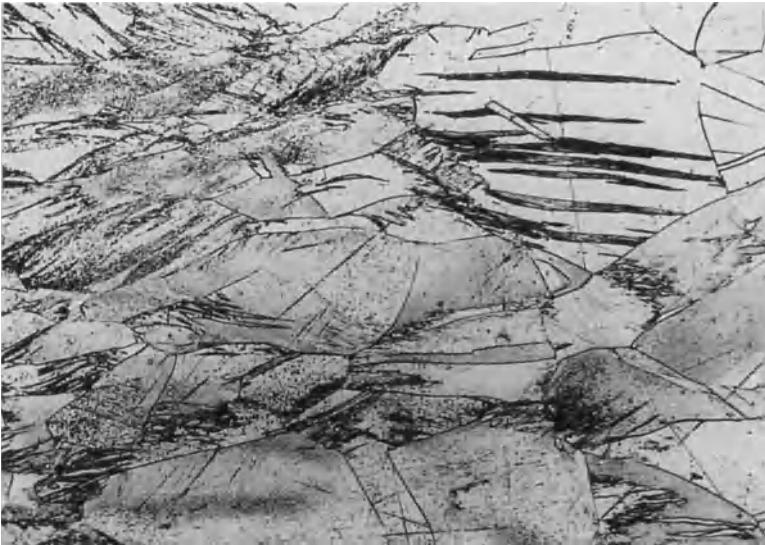
Fig. 8b : Detail of Coin No. 4 with elongated grains and slip traces. Width of view: 1 mm.
