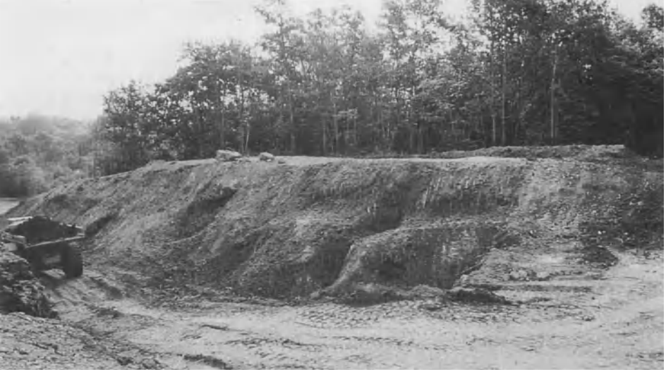
Fig. 11: Benches in the roofwall of the vein at Les Fouilloux.
