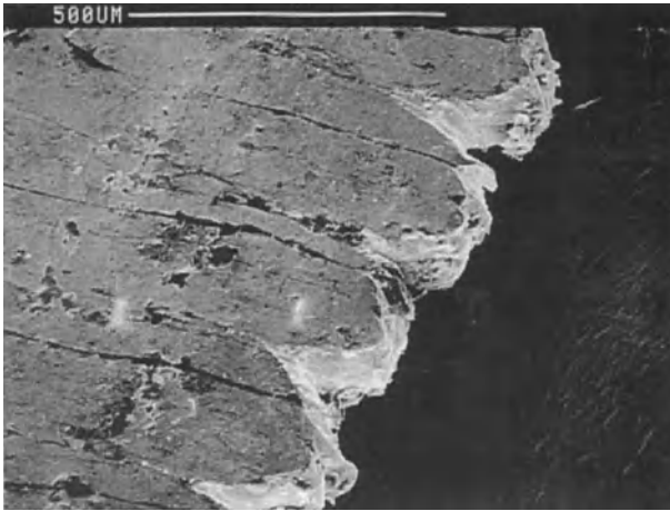
Fig. 20: Scanning electron micrograph showing the edge of a flat wrought wire (modern reproduction), made from an oblique beaded wire. Separations between beads are still visible; parallel black lines are the remains of the original separations from before hammering.
