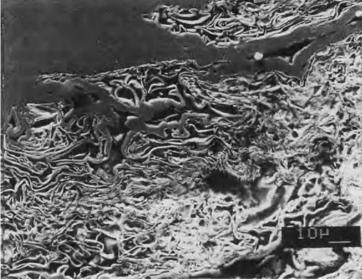
Fig. 2: SEM-photo of a microsection through a gold grain from the decoration of the Big Dish, Varna.
