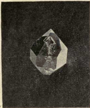
Crystals showing Large Cavity containing Liquid, Movable Bubble and Movable Rhomb of Calcite.
