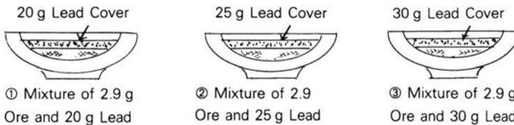
Figure 12.21. Scorification assay, third step: combining ore and lead and covering with lead
