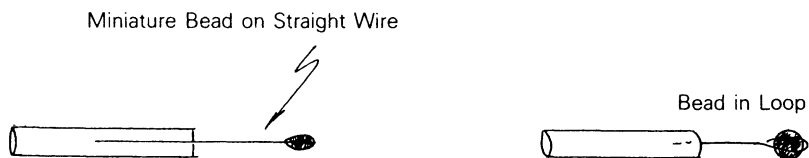
Figure 3.17. Beads formed in a loop and on a straight wire
