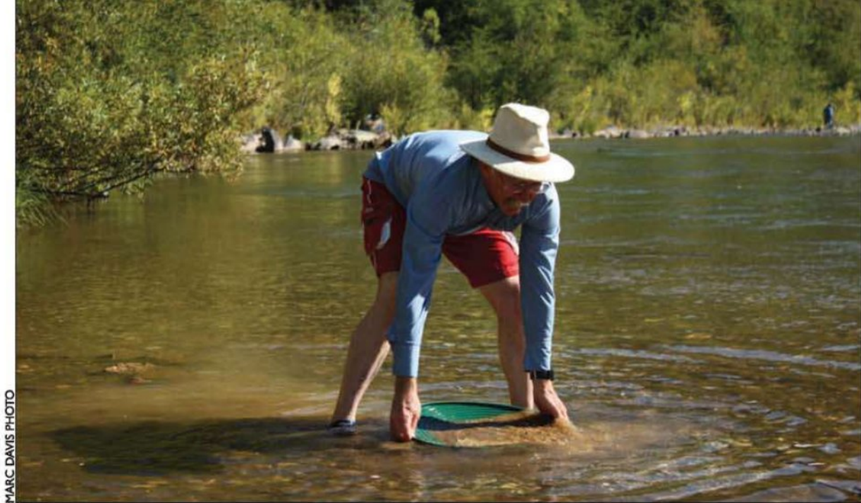
I found that the Australian competition pan works well in calm water, but could not handle swifter moving currents in other parts of the river.
