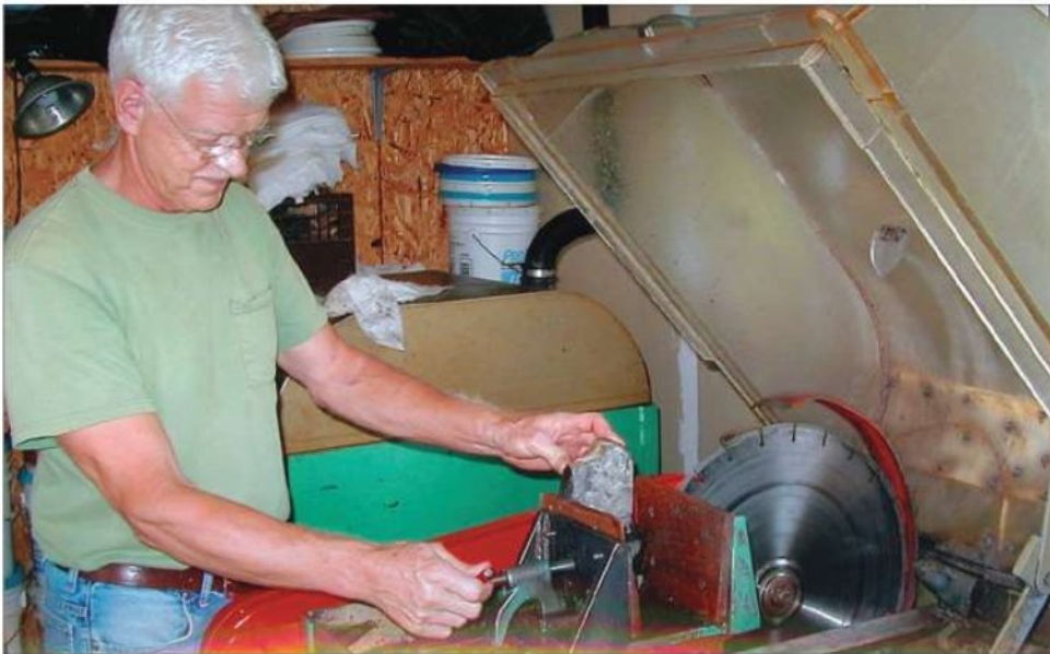
In his workshop, Roy has a number of Highland Park slab saws ranging from 18 to 24 inches in diameter.
