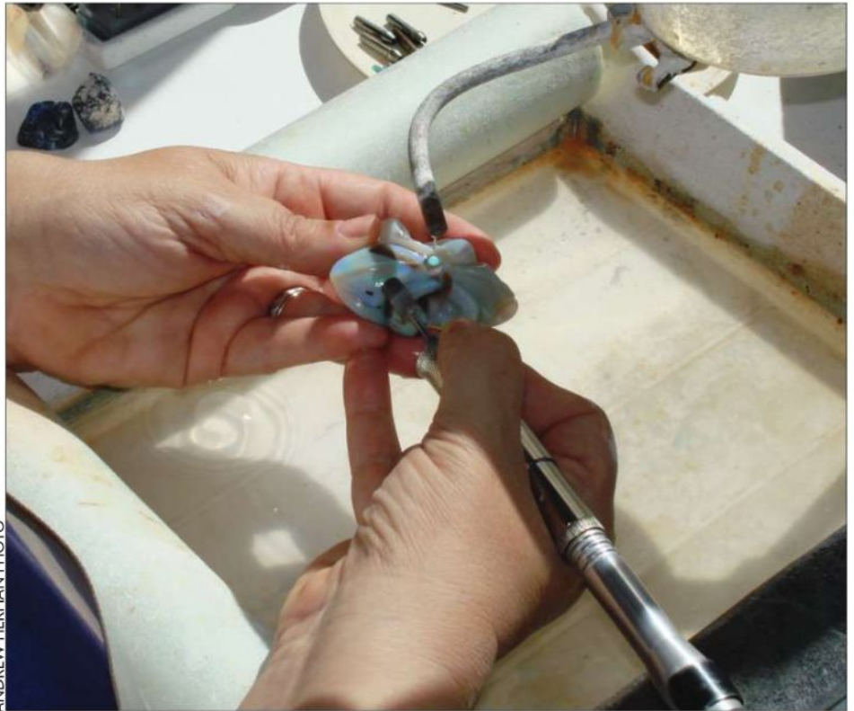
Helen creates her gemstone carvings with a hang-up-style Foredom flexible shaft tool, which has a thin handpiece that she holds like a pen.
