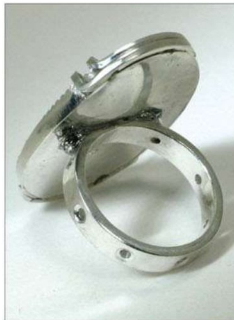
Use the bezel pusher to tighten the bezel wire against the stone.
