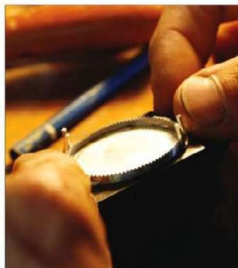
Using pliers, bend the right ends of the prong wires back so that they stick up from the table.
