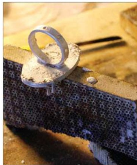
Filing a flat spot over the soldered joint of the ring provides a larger area of contact for soldering.
