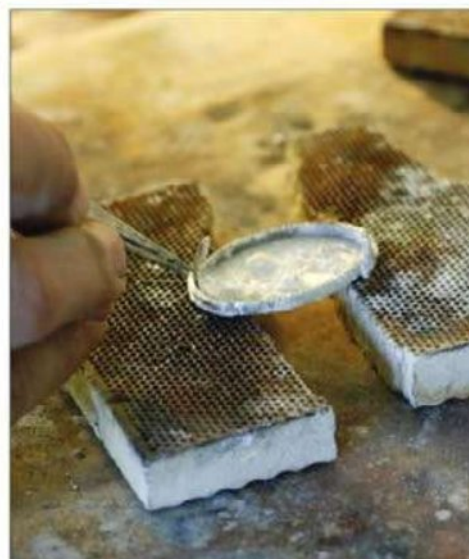
During soldering, the flux will bubble. Use the pick to push things back into place.
