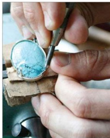
Use the bezel pusher to tighten the bezel wire against the stone.
