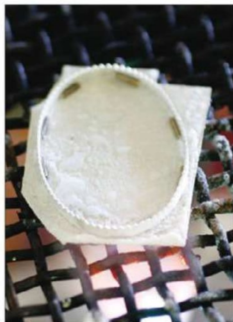
When soldering the bezel to the backing plate, use a metal mesh platform so you can heat the piece from above and below.
