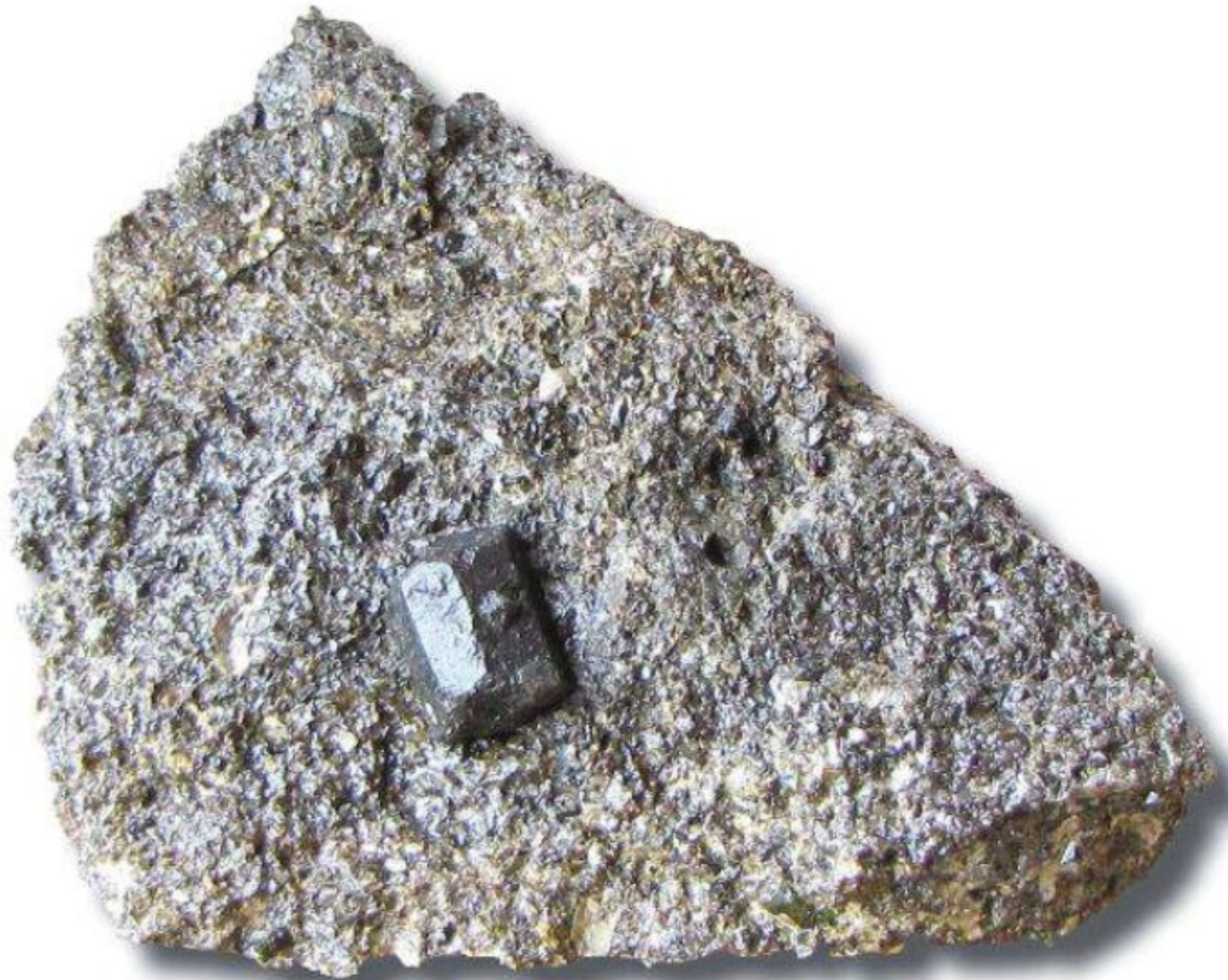
A large augite crystal is sticking half out of its fine-grained lithic tuff matrix.
