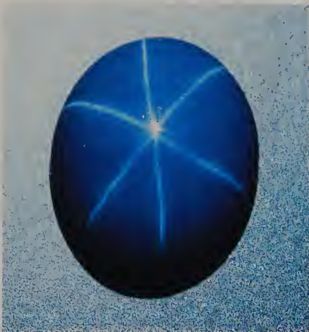
Fig. 14.10 A synthetic star sapphire. Note how long and sharp the rays of the star are.
