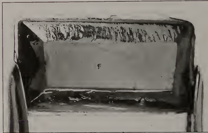
Fig. 12.14 A typical glass stone—rounded facet edges, orange-peel like surface, a bubble in the center, simple cutting style with just five crown facets
