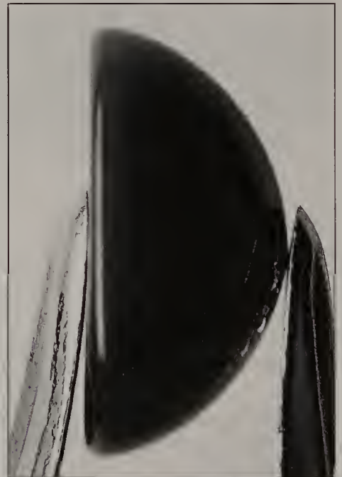
Fig. 14.11 Side view of a synthetic star sapphire with a flat base. Note how opaque and symmetrical it is.
