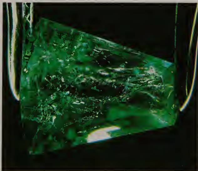
Fig. 8.35 Same emerald in darkfield illumination. A lay person might think this is a reject when in fact, it's a good emerald. The white rectangular areas along the edge are light reflections.
