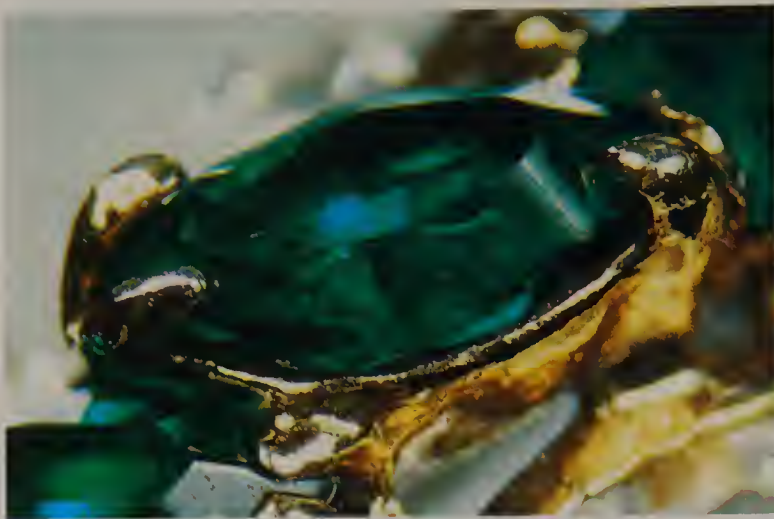
Fig. 12.11 Concave facets and a rounded girdle and facet edges are evidence this is a glass stone.
