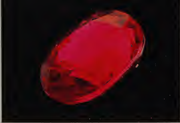
Fig. 12.5 When the ruby is rotated 45°, light shines through it. This is typical behavior of corundum and emeralds but not of stones like glass and garnet.
