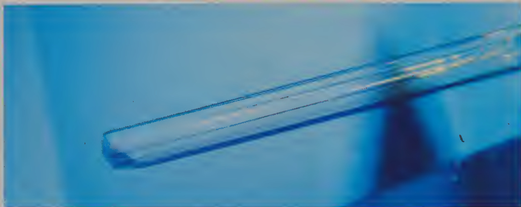
Fig. 8.3 Pargasite crystal in a Kashmir sapphire. Photo from Gübelin Gem Lab.
