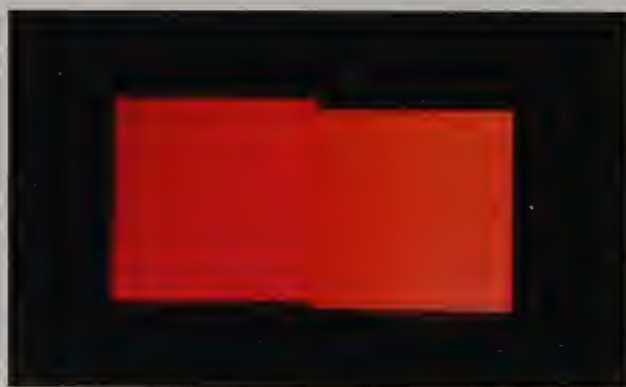
Fig. 12.8 Thai ruby dichroism in a calcite dichroscope. Photo by C. R. Beesley of AGL.
