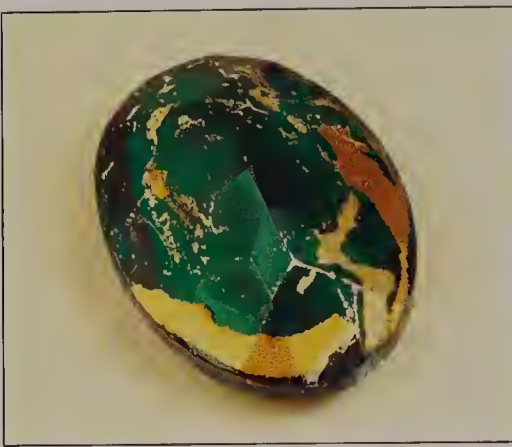
Fig. 12.18 Bottom of a glass stone that has lost most of its foil backing.
