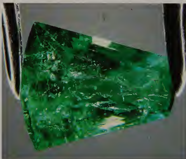
Fig. 8.36 The emerald does not look any better when the background is changed to a light color. The light coming up diagonally through the stone still exaggerates the flaws.
