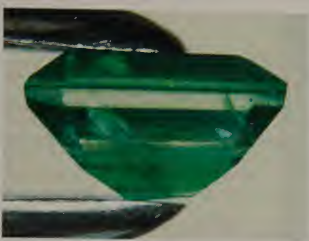
Fig. 12.20 Side view of a colorless-beryl triplet. A dark green line is visible around the girdle where the two parts of the stone have been joined with a colored cement.
