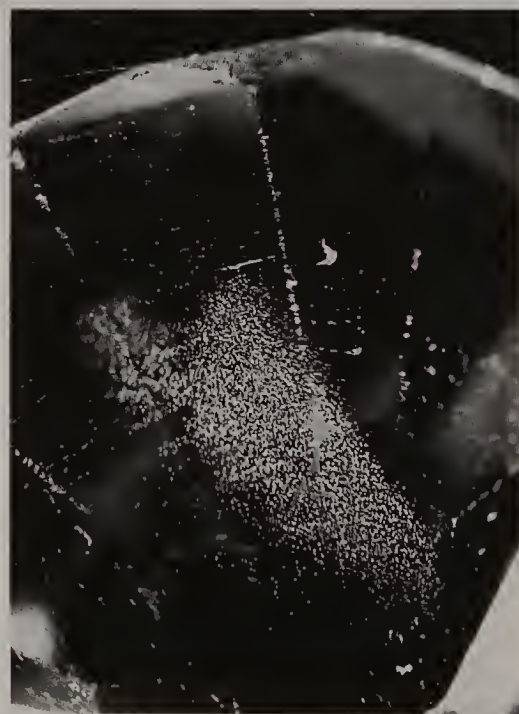
Fig. 13.6 A cloud of tiny gas bubbles in synthetic ruby
