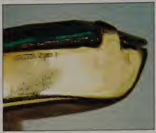
Fig. 12.19 Sometimes foil backings are visible on stones set in closed back mountings.
