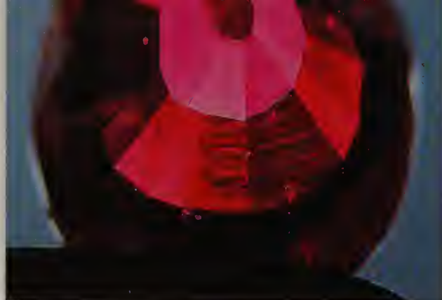
Fig. 13.3 Pavilion of a mixed-cut natural ruby, tilted to show the pleochroic purple and orange-red colors. The jagged curved lines are not synthetic growth lines.
