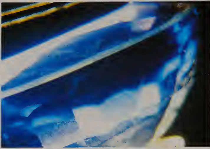
Fig. 12.24 Profile view of a sapphire doublet. Note the separation line where the top and bottom of the stone were joined. Photo from the Asian Institute of Gemological Sciences (AIGS).
