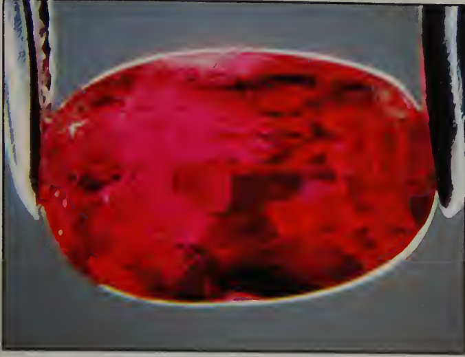
Fig. 8.37 A Thai ruby with an acceptable clarity viewed under darkfield illumination.
