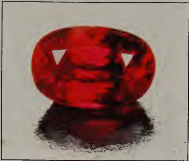
Fig. 8.38 Same ruby viewed with overhead lights. The "fingerprint" inclusions visible in figure 8.37 are hardly noticeable.
