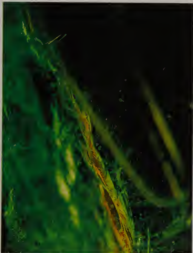
Fig. 11.3 Yellow-orange color flashes in the filled fractures of an epoxy-treated emerald. When these emeralds are tilted so the background becomes lighter, the flashes may disappear or turn blue. Photo courtesy AIGS; photo by Gary Du Toit.
