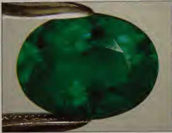
Fig. 8.29 An emerald with a serious crack across it viewed in normal overhead lighting.
