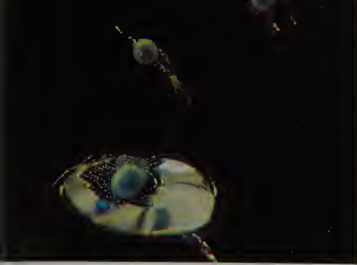
Fig. 8.12 "Snowball-like" cores with a radiating glassy fracture and lacy fringe in a heat-treated sapphire. Photo by C. R. Beesley of AGL.
