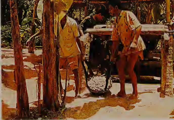
Fig. 2.3 Basket hopefully full of gem-rich clays and gravels. The contents will be put in a larger basket in a shallow reservoir where Sri Lanka miners will wash away the clays, leaving heavier minerals and hopefully some gems. Photo by Cynthia Marcussom, Cynthia Renée Co.
