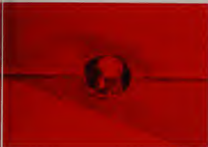
Fig. 8.14 "Saturn-like" inclusion with flattened spherical core in twinning plane. Photo by C. R. Beesley of AGL.
