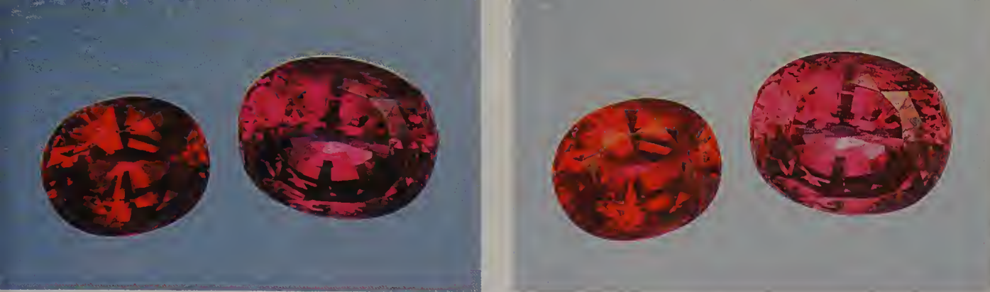
Figs. 5.2 & 5.3 Two photo exposures of a Thai ruby (left) and a Sri Lankan pink sapphire (right), as identified by Los Angeles dealer Andrew Sarosi. Note how the color looks redder and the extinction areas become blacker when the tone is darker. The actual pink sapphire has a rich "hot pink" magenta hue that makes it look distinctly different from the ruby. (Keep in mind that the printing and developing processes usually alter the true color of gems in photos.) Most Asian dealers identify pink corundum stones as rubies.
