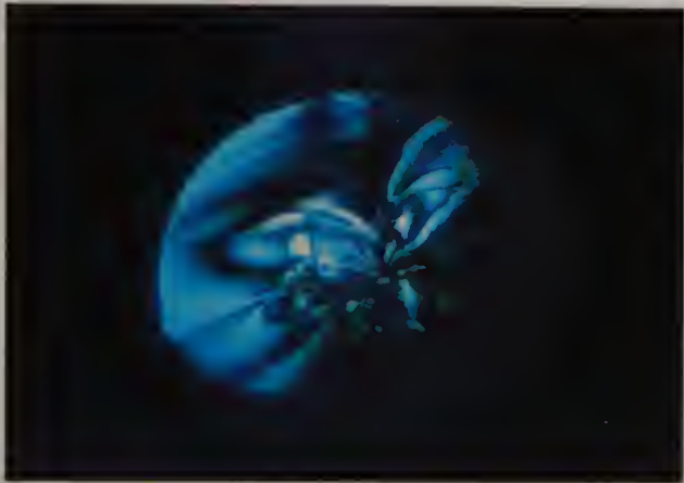
Fig. 10.5 A classic, highly reflective, circular fracture, typically found in heat-treated sapphire. Photo by C. R. Beesley of AGL.
