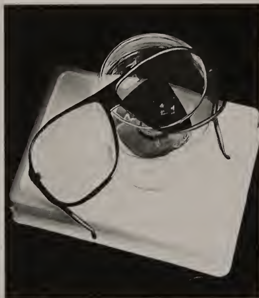
Fig. 12.6 Stone viewed through a home-made polariscope—a wine glass and the lenses of a cheap pair of Polaroid sunglasses
