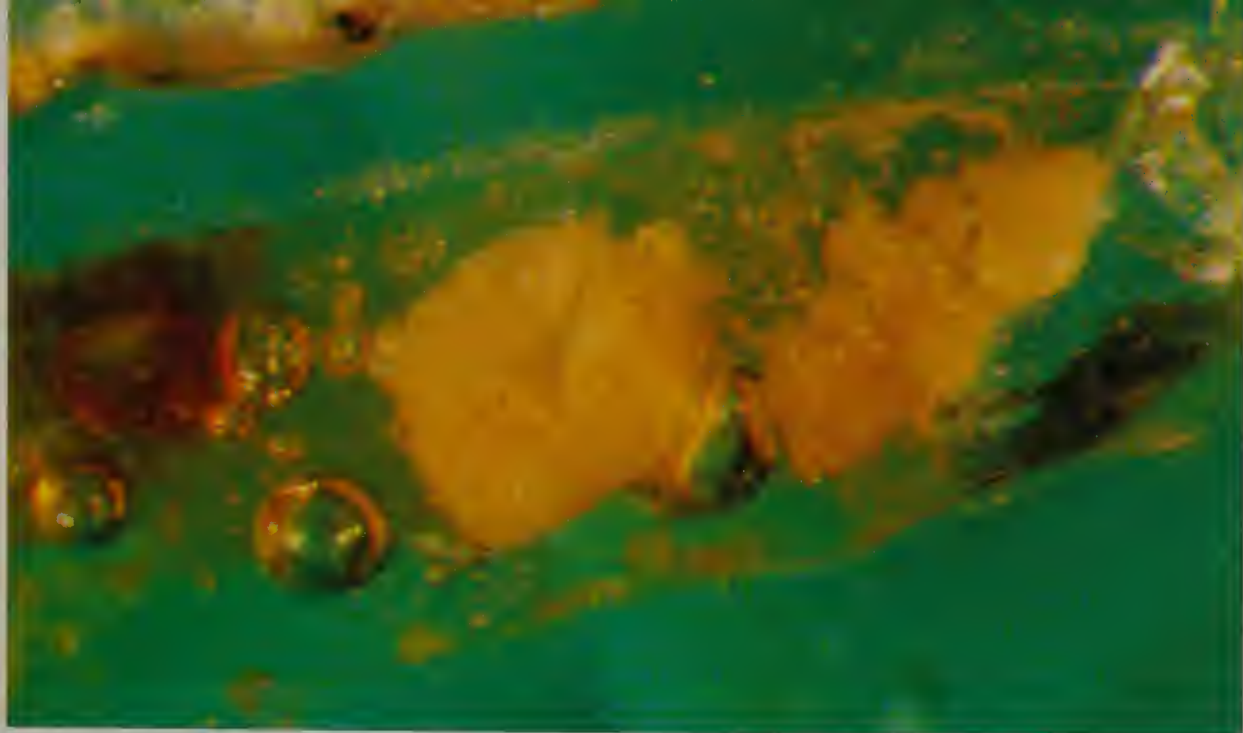
Fig. 11.2 Residue and trapped air bubbles in a fracture of an epoxy-filled emerald. Photo courtesy AIGS (Asian Institute of Gemological Sciences); photo by Gary Du Toit.
