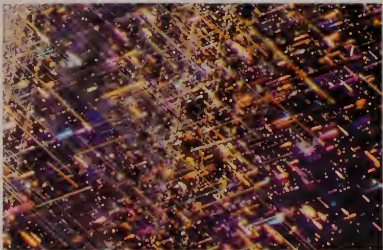
Fig. 8.4 "Silk" in sapphire. Photo from Precious Link.
