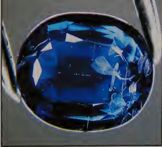
Fig. 8.39 Sapphire with an acceptable clarity and good transparency. The flaws in this stone look white when viewed in darkfield lighting. They're colorless and hardly noticeable under overhead lighting.
