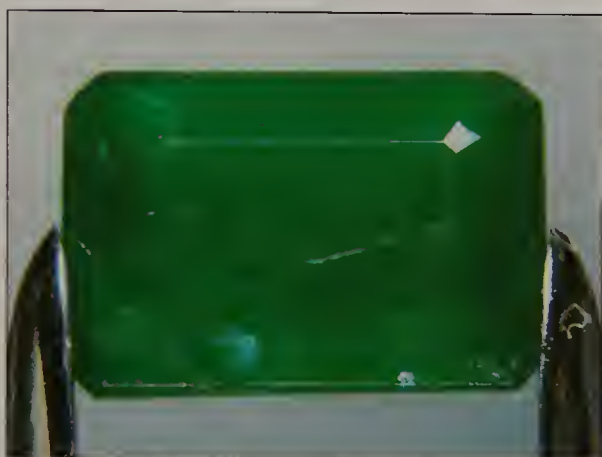
Fig. 8.27 A translucent emerald in overhead lighting. The surface cracks are not noticeable to the unaided eye.
