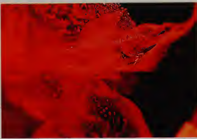
Fig. 13.13 Veils and fingerprint inclusions in a Kashan flux synthetic ruby. Photo by C. R. Beesley of AGL.
