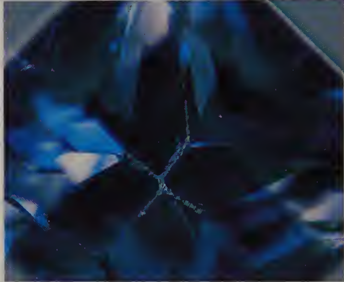
Fig. 8.19 Abraded pavilion facets which are visible through the table of this sapphire
