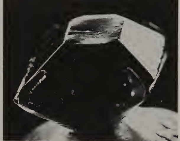
Fig. 12.10 The concave table facet and the rounded facet edges are sure signs this is a glass stone. Note, too, how the crown has only 5 facets.
