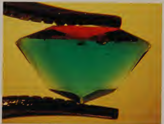
Fig. 12.23 Side view of a heat-fused garnet and glass doublet in water. Face-up it resembles an emerald. Photo by Alan Hodgkinson.
