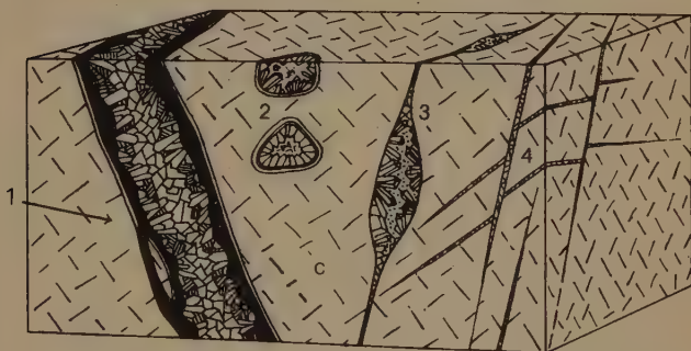
13 Block diagram illustrating an ore vein, druses, and alpine fissures. 1, Ore vein; this hydrothermal vein is symmetrically lined by ores (black and shaded) and filled with gangue minerals (white), such as quartz and calcite. Along the contact with the country rock there is an alteration zone. Veins may vary from a few cm. to several metres in thickness. 2, Druses, irregular to rounded cavities with crystals lining the walls. 3, Alpine fissures: thin cracks in the rocks widen to large cavities with room for free-standing crystals to grow in. 4, Crevices, a few mm. to a few cm. wide, often occurring in swarms: usually filled with quartz or calcite. c, Country rock.
