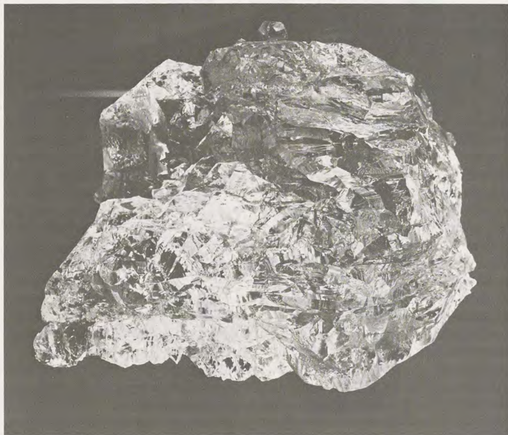
Fig. 9-23 A completely etched mass of morganite from Brazil measuring approximately 16 \times 12 \times 12 cm ( 6\frac{5}{16} \times 4\frac{3}{4} \times 4\frac{3}{4} in). The orientation is with the c -axis vertical; there are numerous hexagonal "trumpet" etch pits on both ends of this axis. Jeff Kurtzeman photo.
