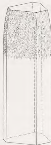
Fig. 9-7 Beryl crystal with tapered and etched termination, showing overdevelopment of alternate faces of the prism m\{10\bar{1}0\} .
