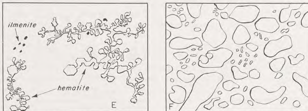
Fig. 10-3 Typical inclusions in beryl. E: Extremely thin plate-like dendrites of ilmenite (black) and hematite (orange) grown upon the basal plane c\{0001\} of aquamarine from Brazil. F: Extremely thin voids resembling flattened bubbles forming planes of inclusions parallel to the basal plane c\{0001\} ; as in E, some are epitaxial; all are so thin that vivid colors arise from those which interfere with light. From V. G. Feklichev, Berill: morfologiya, sostav i struktura kristallov . (Moscow: Izdatelstvo Nauka, 1964) and E. Gübelin, Internal World of Gemstones: Documents from Space and Time (Zurich: ABC Edition, 1973).
