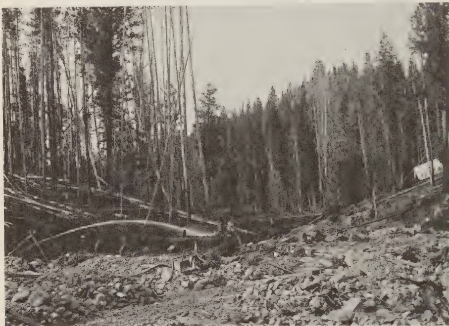
FIGURE 110. Washing gravels for sapphires on the West Fork of Rock Creek southwest of Phillipsburg, Montana. Barren topsoil is washed away by hose to expose sapphire-bearing gravels beneath. Large pebbles and boulders are moved out of the way to gain access to the lowest layers of gravel resting on bedrock. Courtesy U. S. Geological Survey.
