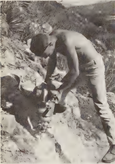
FIGURE 20. Atlas-Copco portable gasoline motor drilling machine in operation. This unit is entirely self-contained. It weighs slightly over 50 pounds and is easily transported and operated in the field. Photograph taken at the Hercules Mine, near Ramona, California.
