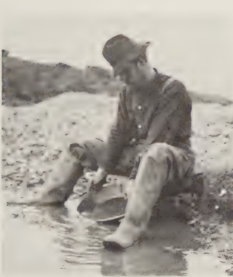
FIGURE 17. A "sourdough" demonstrating the final stages of gold-panning on Boulder Creek, Alaska. Only a handful of small gravel and sand now remains in the pan, plus whatever flakes and nuggets of gold have been concentrated. Courtesy U. S. Geological Survey.
