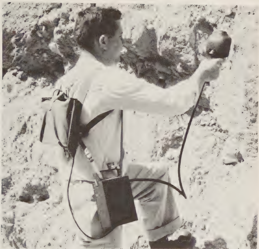
FIGURE 122. Battery-powered ultraviolet light rigged for field work. This photo was necessarily taken in daytime to show all features of the equipment. Courtesy Ultra-Violet Products, Inc., San Gabriel, Calif.
