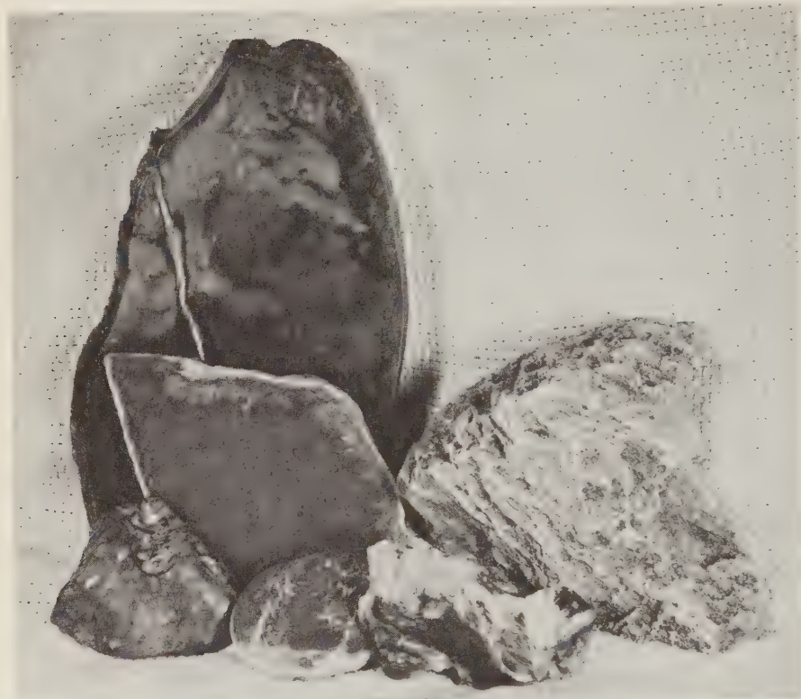
FIGURE 119. North American nephrite specimens. The large slab in the background is dark green Alaskan jade showing several streaks of chatoyant grayish-green material near the top. Leaning against it is a slab of Wyoming nephrite showing a rind of altered material and small black specks scattered throughout the bright green unaltered material within the core. On the right is a rough partly altered specimen of similar material. The lower left and lower right specimens are also from Wyoming while the rounded pebble in the center is from a beach deposit in Monterey County, California.
