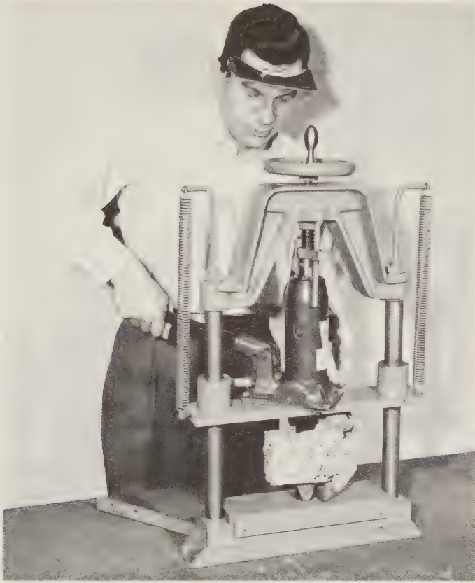
FIGURE 124. An extremely effective rock-trimmer utilizing a hand-pumped hydraulic jack for its motive power. Note that the operator is wearing a heavy leather mitt to protect the hand holding the specimen and plastic goggles to protect the eyes from flying chips of rock when the specimen parts in two. Courtesy Ward's Natural Science Establishment, Rochester, N. Y.
