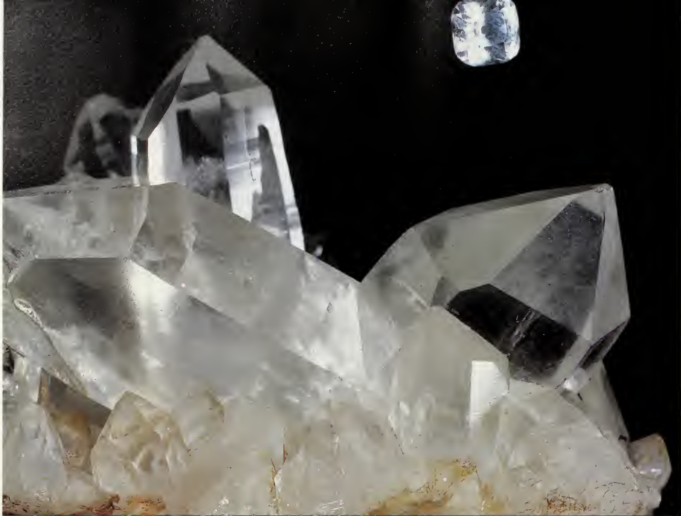
Quartz crystals twinned at right angles according to the Japan Law, from Kurasawa, Kai Province, Japan.
