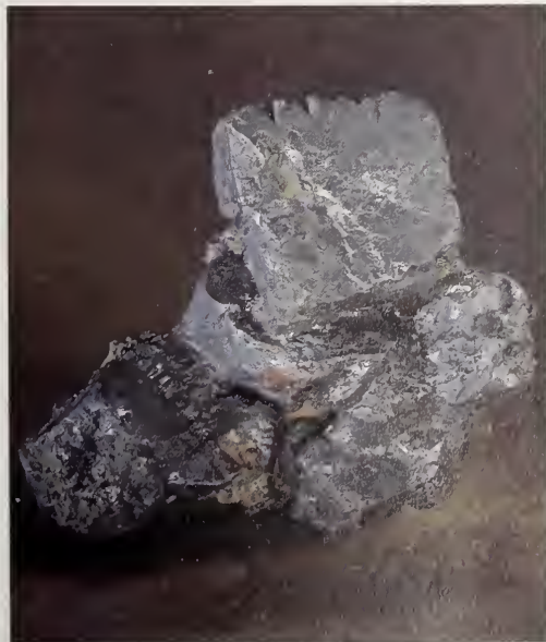
This silver sulfide specimen from Johanngeorgenstadt, Saxony, Germany, originally crystallized as the high-temperature isometric polymorph argentite. On cooling, it underwent internal reorganization to become the monoclinic polymorph acanthite, but retained its original external form.
