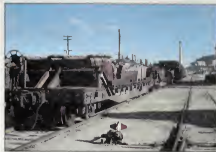
These raw copper ingots were cast in the form of anodes at the smelter at the Ajo copper mine in Arizona. At a refinery, they will be dissolved in an electrolytic solution, through which the copper ions will pass to accrete onto a copper cathode as the pure metal. Impurities dropping to the bottom of the vat will then be further processed for gold, silver, platinum and other valuable metals. (Dennis Cox, United States Geological Survey.)
