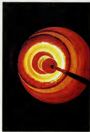
A boule of synthetic ruby being created using the Verneuil Process. Gemstones cut from this artificial crystal will be almost identical to natural rubies.
