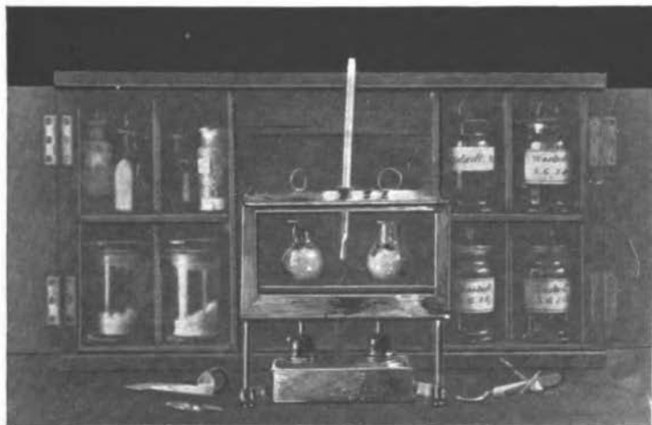
CABINET OF SPECIFIC GRAVITY SOLUTIONS.
