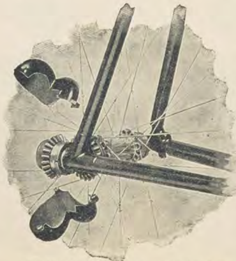
Rear Hub of "Sterling" Chainless with Gear Cases removed.
