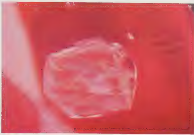
Plate 1. Microscopic examination of the interior of gemstones can reveal clues to their origin. Characteristic of Burmese rubies are crystals of calcite which can be recognised by their marked cleavage planes. Where such crystals are present it is a pretty foolproof guide that the stone is not only natural but also from Burma. (Magnification x 25.)
