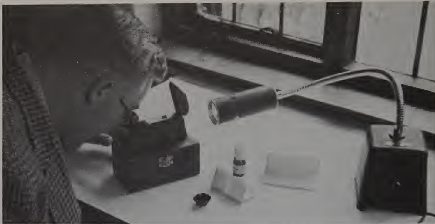
One way of testing gems is to measure their light-bending power with an instrument called a refractometer, which the better jewelers have in their shops. Not all gems can be checked with it.
