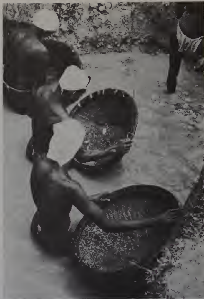
(Left) In some areas of Sri Lanka (Ceylon) there are gravels about 30 feet (9 meters) below the surface containing ruby, sapphire, garnet, topaz, zircon, tourmaline, spinel and many other gems except diamond. They are mined by making shored pits and winching up gravel baskets filled by men below. (Right) The sandy gravel is washed and swilled in these baskets to remove the sand and lighter elements so that the precious stones, which are generally heavier, remain and can be picked out.
