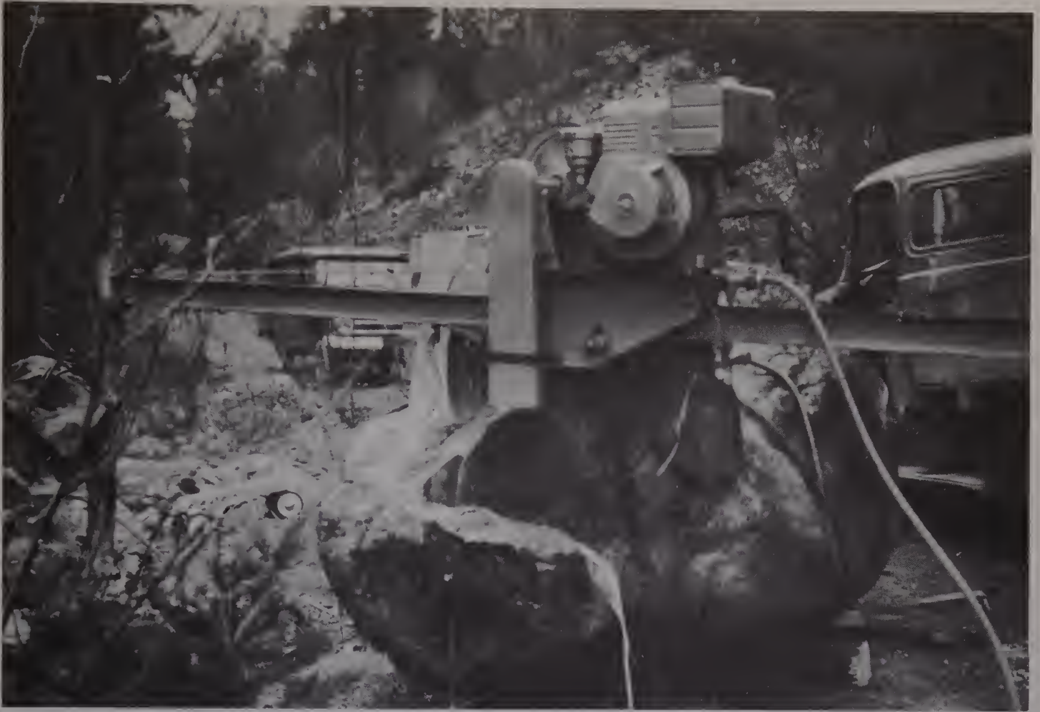
Jade is found in the form of boulders. In this picture a portable saw is being used to make a test cut on a boulder found along Bridge River in British Columbia to assess its value.
