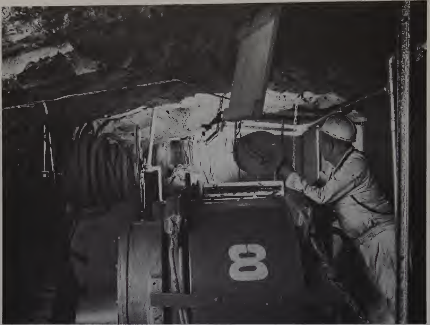
Some diamonds are mined from a thousand feet or more underground by cutting into the pipes of a rock called kimberlite in which the rough diamonds were brought towards the surface from about 120 miles down. A cave is cut in the kimberlite and as the roof caves in the broken rock is dragged out by scrapers like this in the Bultfontein Mine, Kimberley, and hauled to the surface for extraction of diamonds.
