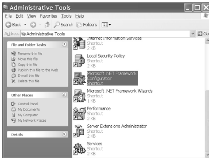
Figure 16-4 The Microsoft .NET Framework Configuration applet provides access to the security policy management capabilities of .NET.
