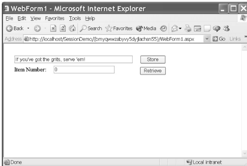
Figure 15-8 The session identifier passed as part of the URL in a cookieless session
