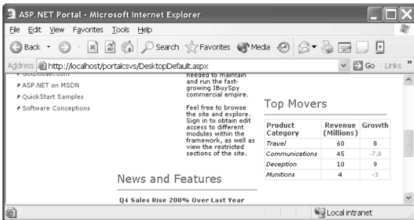
Figure 14-6 The Top Movers section created using an XML document containing data and an XSL/T document describing the appearance
