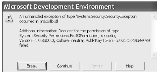
Figure 16-6 A System.Security.SecurityException because the consumer application calling MyFile.Delete did not have FileIOPermission to perform the requested operation
