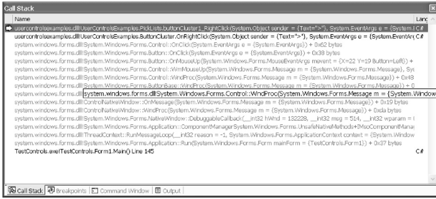
Figure 8-2 The Call Stack shows that the constituent control responded to the event first and that the event is bubbled up to the containing control.
