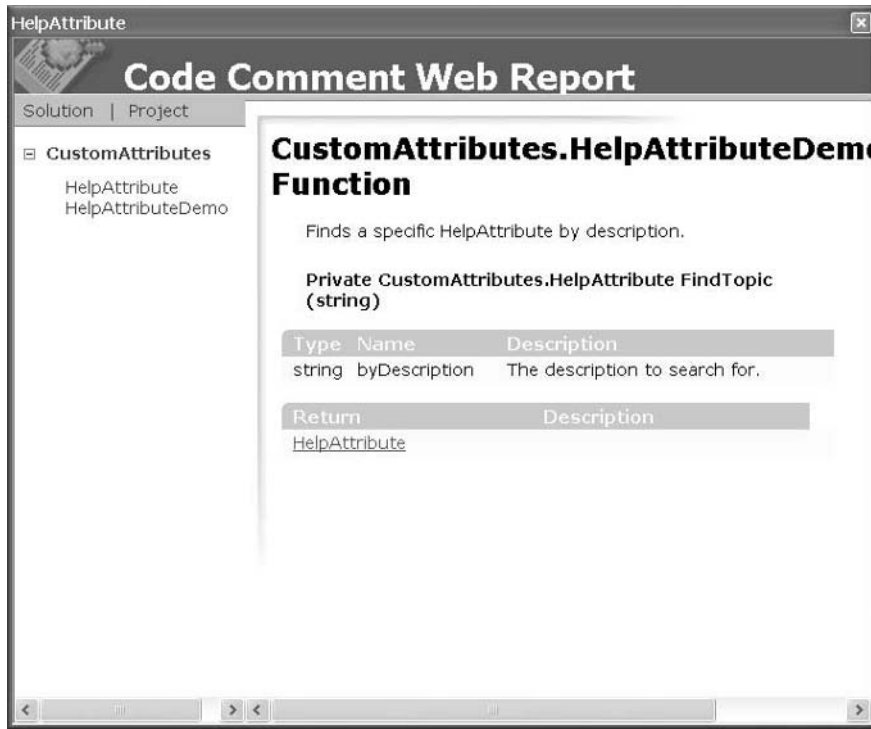
Figure 10-2 The parameter type and name and return type of a method added to a Code Comment Web Report using the <param> and <returns> tags
