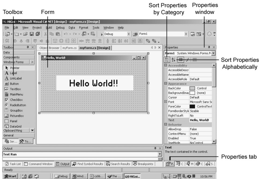
Figure 6.9: When you build a Windows project, the IDE changes to add graphical features.
