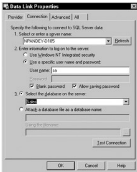
Figure 28-2: Connect to the data source by using the Data Link Properties dialog box.
