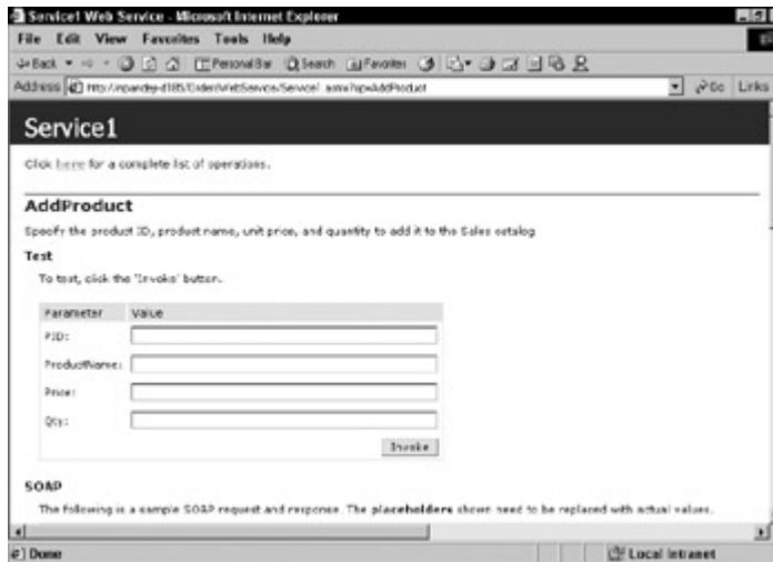
Figure 28-4: Specify the parameters for the AddProduct function in order to test it.
