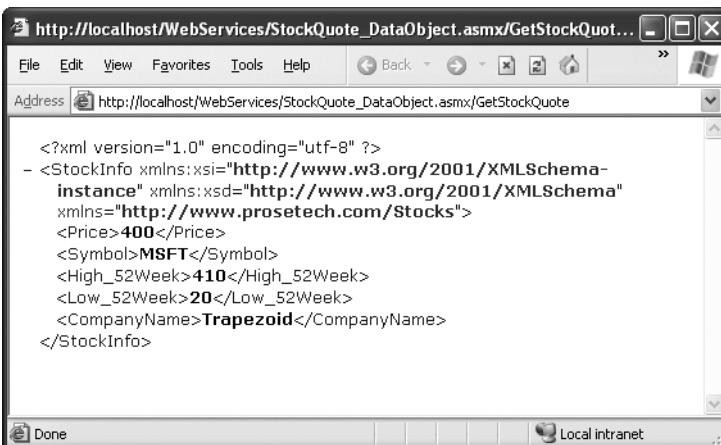
Figure 22-7. The result from GetStockQuote() as a data object
