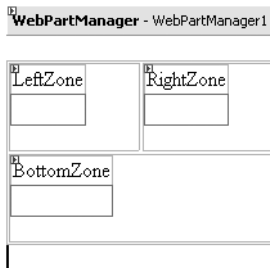
Figure 27-3. A Web Part page showing an HTML table containing WebPartZone controls
