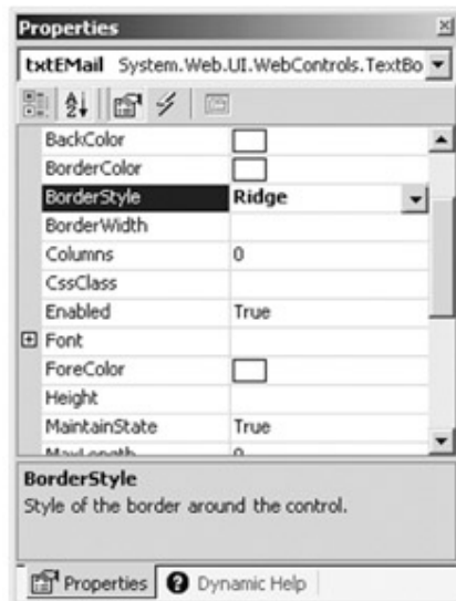
Figure 14-38: Like Windows Forms Controls, Web Form Controls are configured using the Property window
