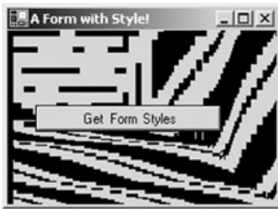
Figure 8-12: ResizeRedraw is a bit off If you set it to "true" you have correct rendering ( Figure 8-13 ).
