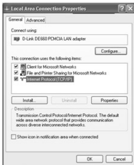
Figure 4.4: The network interface properties, reached through Control Panel Network Connections
