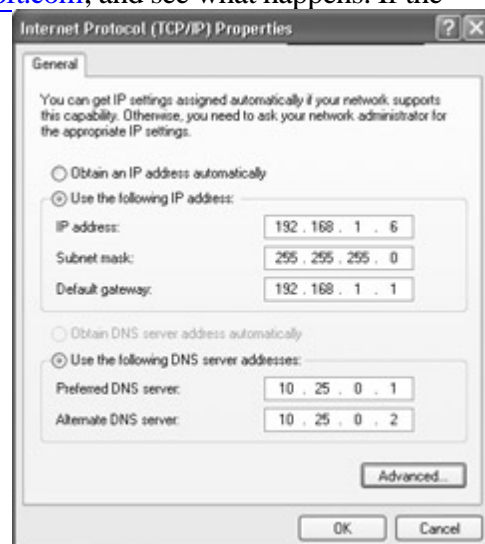
Figure 4.5: The Internet Protocol Properties window in which the DNS server addresses are configured
