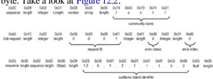
Figure 12.2: Simple SNMP GetRequest packet layout
