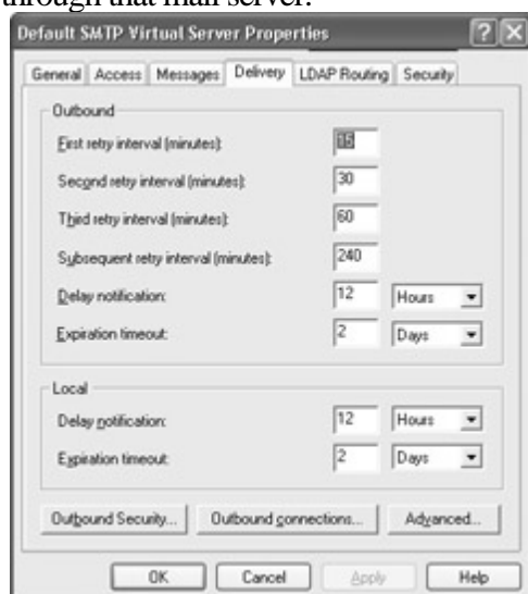
Figure 13.4: The Default SMTP Virtual Server Properties dialog box is where you configure SMTP settings.
