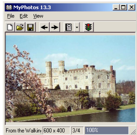
Figure 13.1 Our toolbar will use a raised-button appearance for displaying its buttons. A flat appearance is also possible.
