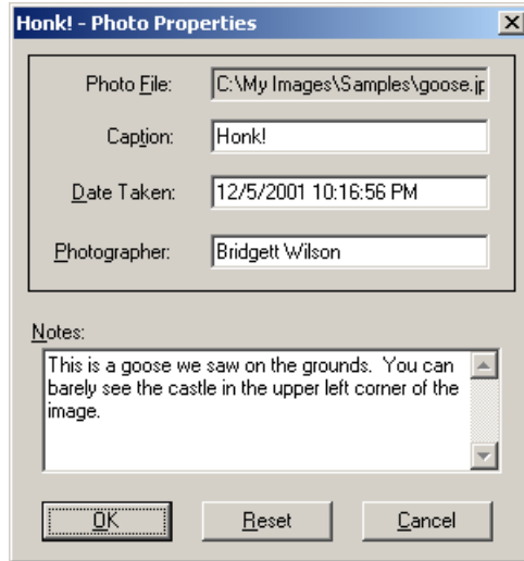
Figure 9.2 Our Photo Properties dialog adds Label and Textbox controls to our inherited form.
