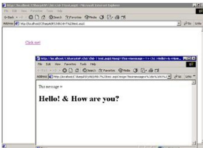
Figure 8.5: Clicking the anchor tag in the leftmost browser causes the second browser to appear and display the message
