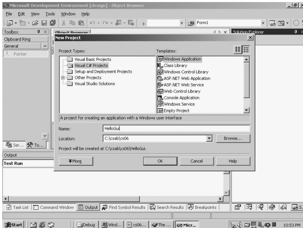
Figure 6.8: You can choose to make a Windows project when you start a new C# project. The editor will continue to load as usual, but the screen will be a little different from what you are used to.
