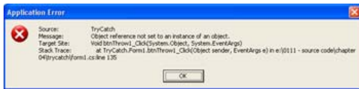
Figure 4.6: The error object contains a wealth of information about the problem with the application.
