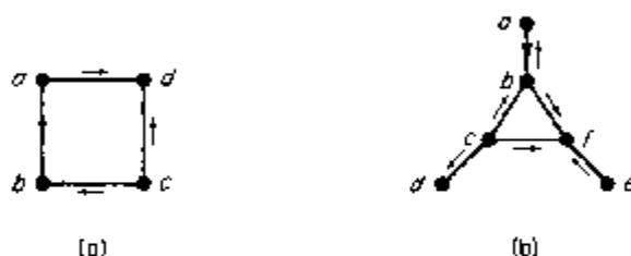
Figure 5.1. Examples of forcing. The arbitrary choice of ab \in F forces the other indicated orientations.
