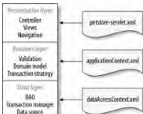
Figure 8-2. The jPetStore application has Spring application contexts to match its three distinct layers
