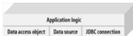
Figure 6-7. Some traditional J2EE applications have application logic that controls implementations of a DAO, a data source, and a connection
