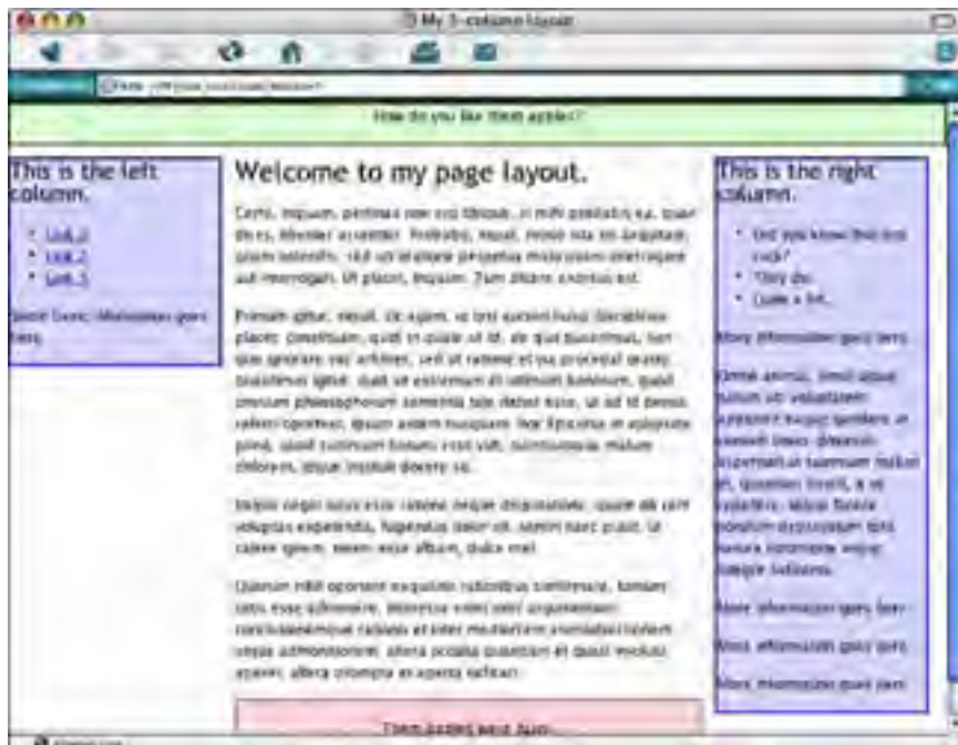
Figure 9-24: Changing the right property of our #right selector to 15 pixels removes the scroll bar, but the positioning is a bit off.
