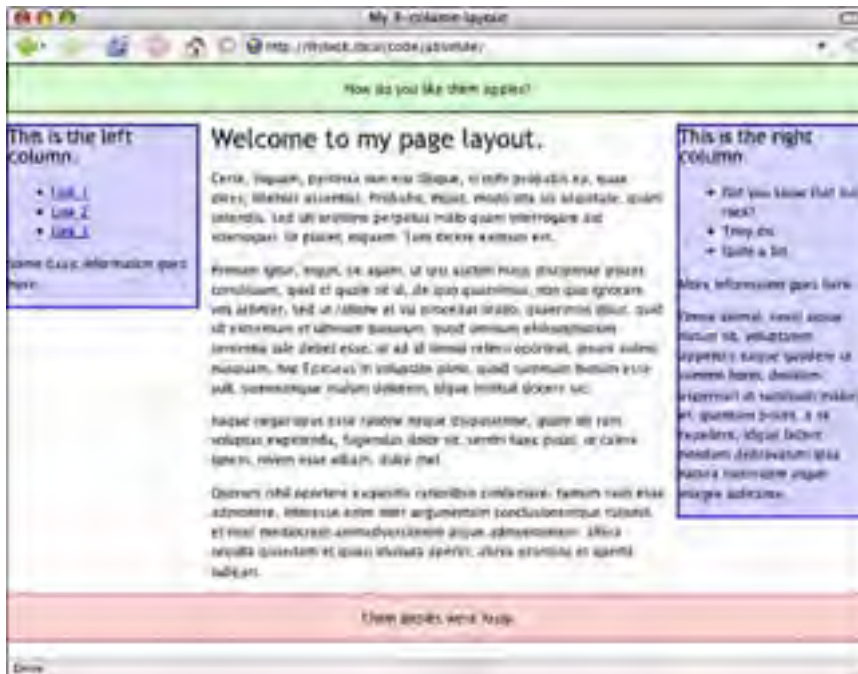
Figure 9-18: By adding padding to the content div that corresponds to the width of the flanking side columns, you can create the illusion of a middle column distinct from those on either side.
