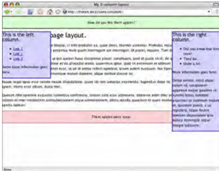
Figure 9-16: With position: relative; applied to your new container block, the left- and right-hand columns' top edges are now contained within their parent. But what about your page's content?
