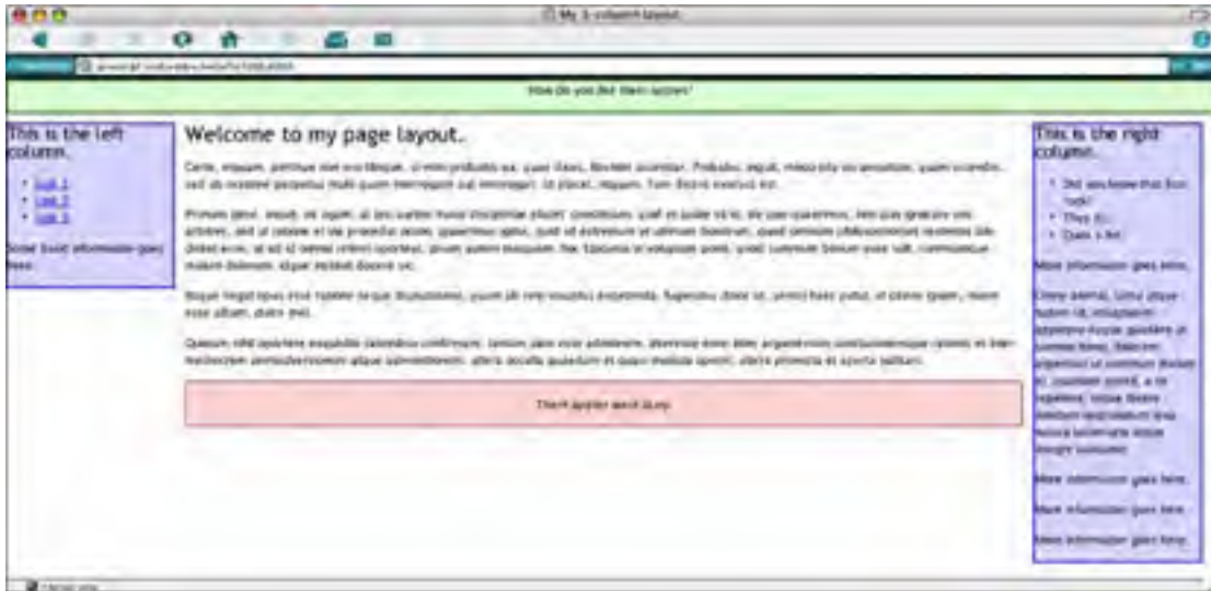
Figure 9-29: In browsers that don't respect the max-width CSS property (such as Internet Explorer on the Mac, shown here), the page layout will simply expand to the width of the window.
