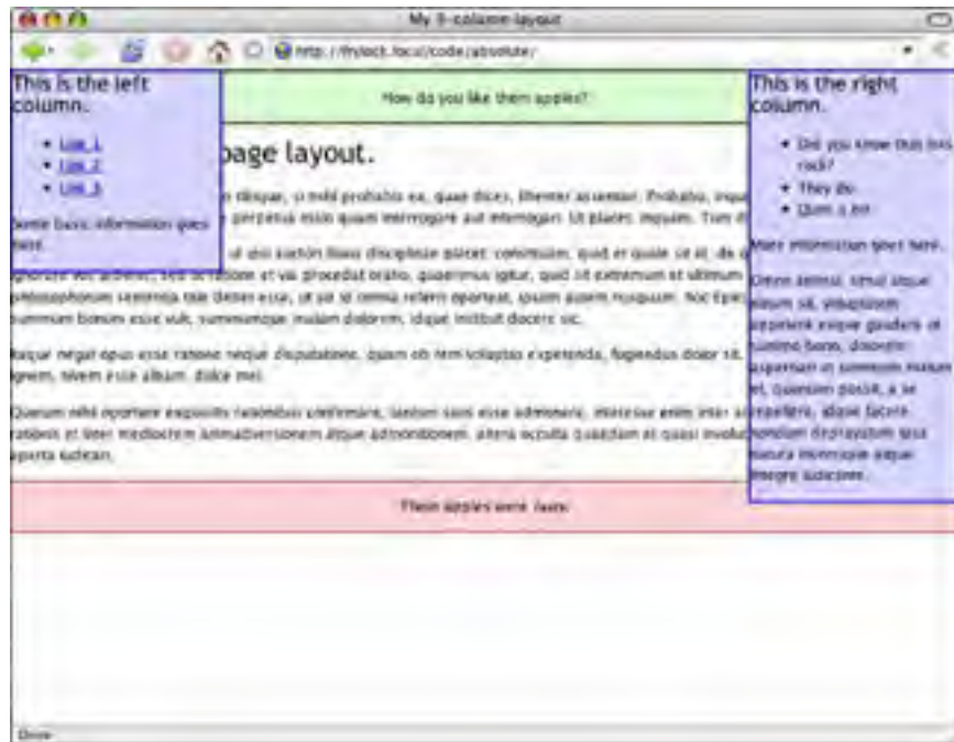
Figure 9-15: Absolute positioning allows you to place the left and right columns — however, you’re not out of the woods yet.
