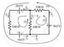
Two unknown currents  $I_1$  (through the 2.00- $\Omega$  resistor) and  $I_2$  (through the 5.00- $\Omega$  resistor) are labeled on the circuit diagram. The current through the 4.00- $\Omega$  resistor has been written as  $I_2 - I_1$  using the junction rule.
