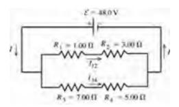
**EXECUTE:**  $R_1$  and  $R_2$  in series have an equivalent resistance of  $R_{12} = R_1 + R_2 = 4.00 \,\Omega$ .  $R_3$  and  $R_4$  in series have an equivalent resistance of  $R_{34} = R_3 + R_4 = 12.0 \,\Omega$ .
