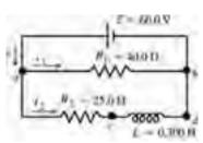
The rate of change of the current through the inductor is limited by the induced emf. Just after the switch is closed the current in the inductor has not had time to increase from zero, so  $i_2 = 0$ .
