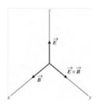
$\vec{E} \times \vec{B}$  must be in the +y-direction (the direction in which the wave is traveling). When  $\vec{E}$  is in the +z-direction then  $\vec{B}$  must be in the +x-direction, as shown in Figure 32.11.
