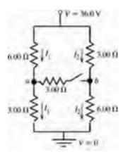
With the switch open there is no current through it and there are only the two currents  $I_1$  and  $I_2$  indicated in the sketch.
