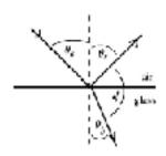
Note:  $\phi = 180.0^{\circ} - \theta_r - \theta_b$  and  $\theta_r = \theta_a$ . Thus  $\phi = 180.0^{\circ} - 54.5^{\circ} - 35.5^{\circ} = 90.0^{\circ}$ ; the reflected ray and the refracted ray are perpendicular to each other. This agrees with Figure 33.28 in the text book.
