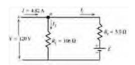
$\mathcal{E}$  is the induced emf developed by the motor. It is directed so as to oppose the current through the rotor.
