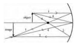
Three principal rays, numbered as in Section 34.2, are shown in Figure 34.5. The principal ray diagram shows that the image is real, inverted, and enlarged.
