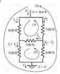
The three unknown currents  $I_1$ ,  $I_2$  and  $I_3$  are labeled on Figure 26.77b.
