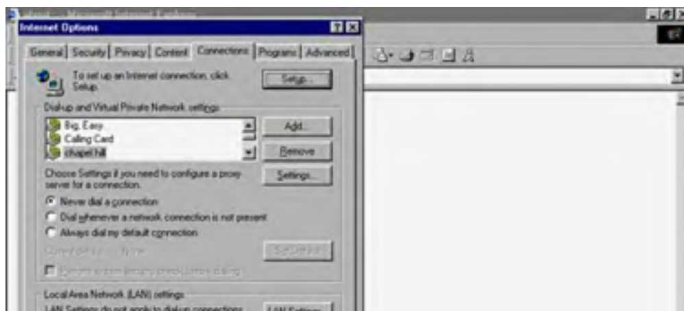
Figure 10.9. Tell your computer that you're on a LAN, so it won't try and connect using your PC's modem.
