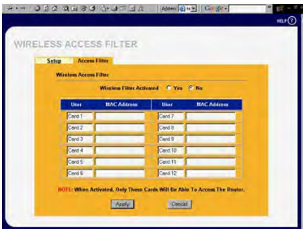
Figure 2.10. You can set your router to only allow access to a network card with a MAC address that you enter.
