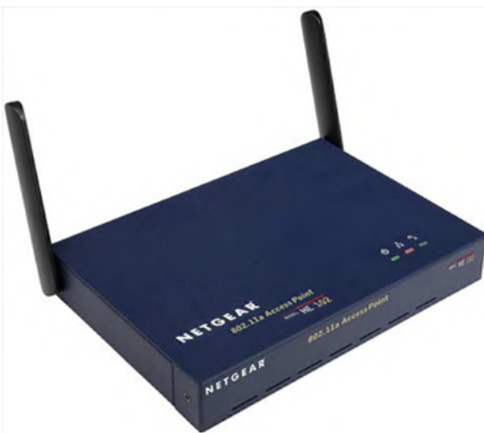
Figure 2.3. This access point includes a built-in router.
