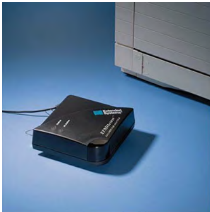
Figure 5.4. An Extended Systems infrared transceiver for printing wirelessly ( www.extendedsystems.com ).
