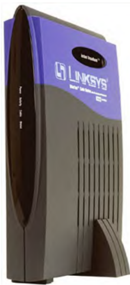
Figure 1.7. A cable modem provides much greater speed for connecting to the Internet than a 56-kilobits per second analog modem.
