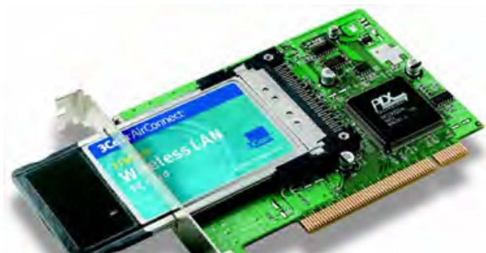
Figure 4.3. A PCI Card wireless network adapter.
