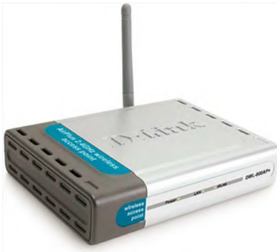
Figure 3.5. This access point from D-Link can be used to connect a cable or DSL modem to provide Internet access to the wirelessly connected computers on your network.
