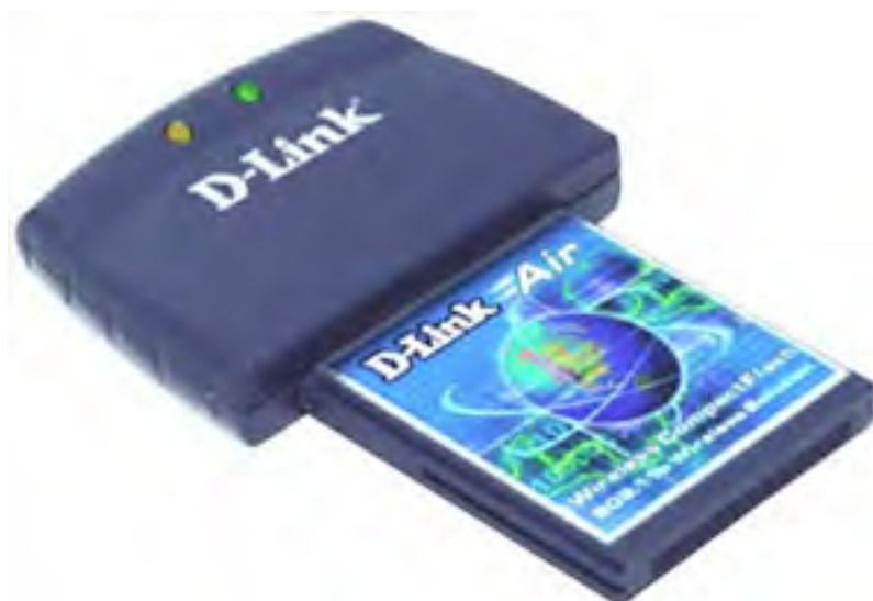
Figure 5.1. You can use a compact flash network card to add your PDA to your wireless network.
