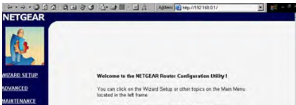
Figure 4.10. Configuring a router by connecting through a Web browser.
