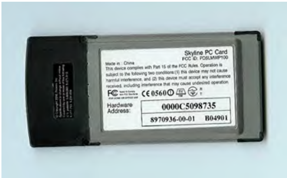
Figure 12.5. Flip your network card over and you should see a clearly marked MAC address.
