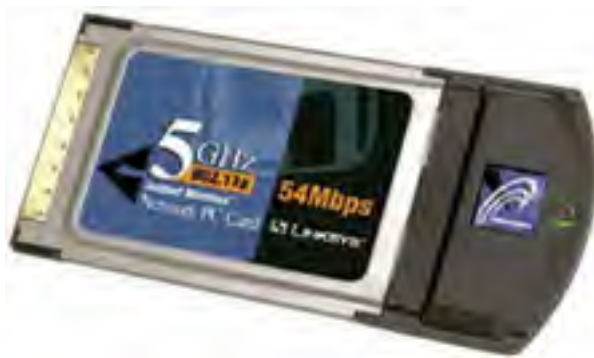
Figure 2.6. An 802.11a wireless network adapter for a laptop.
