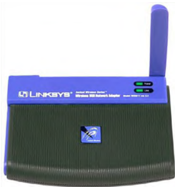
Figure 1.1. A wireless network adapter from Linksys.
