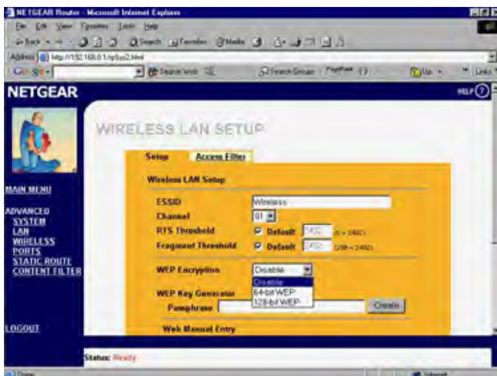
Figure 11.3. Make sure encryption is disabled, or set to the same level at all your computers and at your access point.
