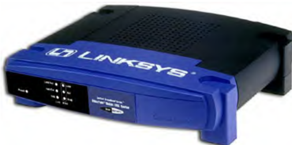
Figure 4.9. You can connect a wired (Ethernet) router, like this one from Linksys, to an access point by Ethernet cable.
