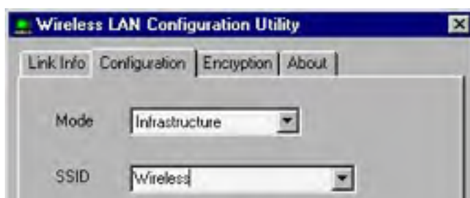
Figure 2.9. Each wireless network adapter needs to provide the same SSID to be allowed access to the network.
