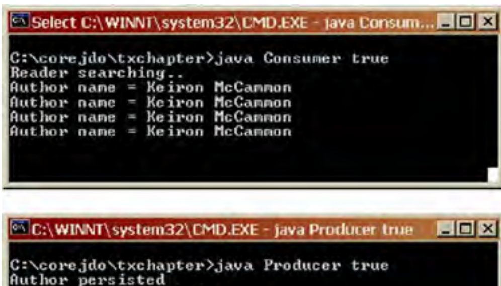
Figure 11-6a and b. The optimistic producer does not lock the data, and the consumer can access it immediately.
