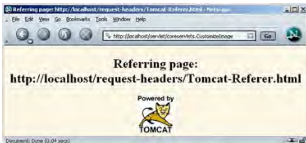
Figure 5-8. The CustomizeImage servlet when the address of the referring page contains neither "JRun" nor "Resin."
