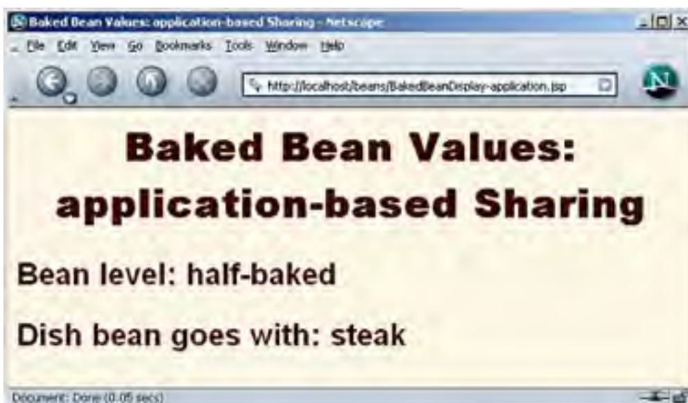
Figure 14-15. Subsequent request to BakedBeanDisplay-application — BakedBean properties persist between requests even if the request is from a different client (as here) or is in a different session.
