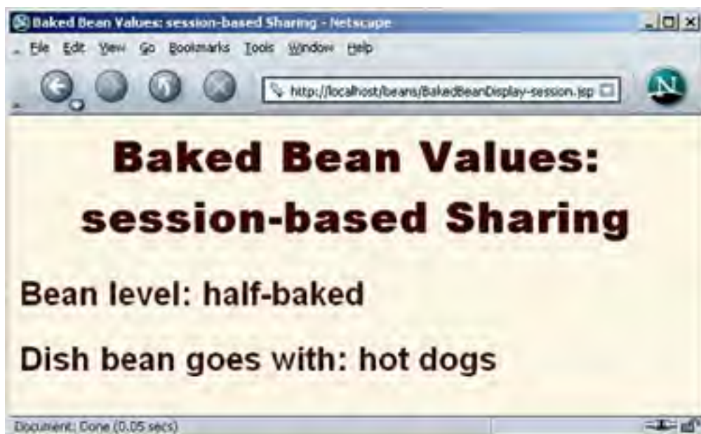
Figure 14-12. Subsequent request to BakedBeanDisplay-session.jsp — BakedBean properties do not persist between requests if the request is from a different client (as here) or is in a different session.
