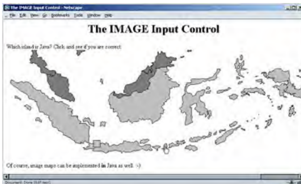
Figure 19-23. Clicking on the image at (447, 272) submits the form and adds map.x=447&map.y=272 to the form data.
