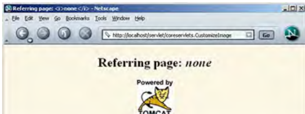
Figure 5-9. The CustomizeImage servlet when the Referer header is missing. When using the Referer header, always handle the case in which the result of getHeader is null .
