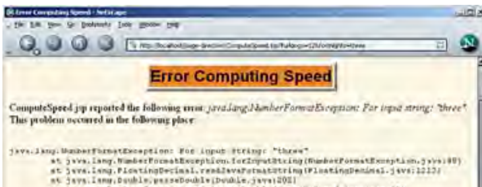
Figure 12-8. ComputeSpeed.jsp when it receives illegal values. Note that the address line shows the URL of ComputeSpeed.jsp , not SpeedErrors.jsp .
