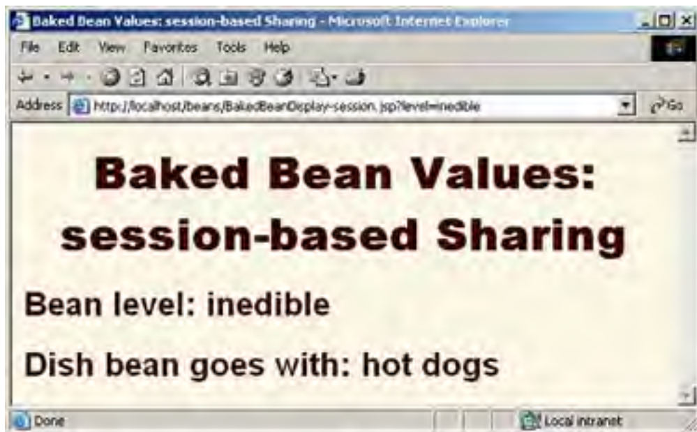
Figure 14-11. Subsequent request to BakedBeanDisplay-session.jsp — BakedBean properties persist between requests if the request is from the same client in the same session.
