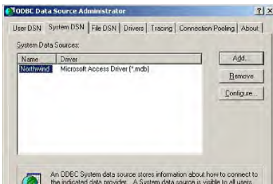
Figure 18-4. Fourth window presented after you have added a new system data source. Click OK to accept the change.
