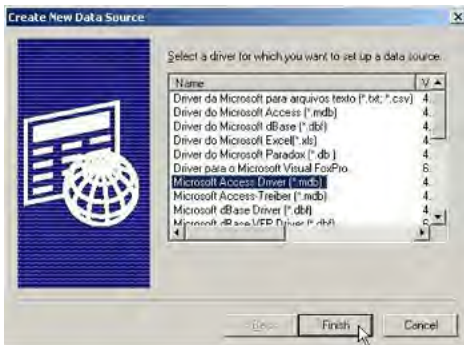
Figure 18-2. Second window presented when you are creating a System DSN. Before continuing the configuration, choose the driver for the data source by clicking Finish.
