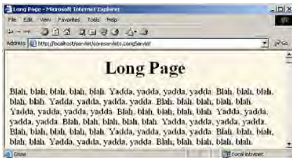
Figure 5-3. Since the Windows version of Internet Explorer 6 supports gzip, this page was sent gzipped over the network and automatically reconstituted by the browser, resulting in a large saving in download time.
