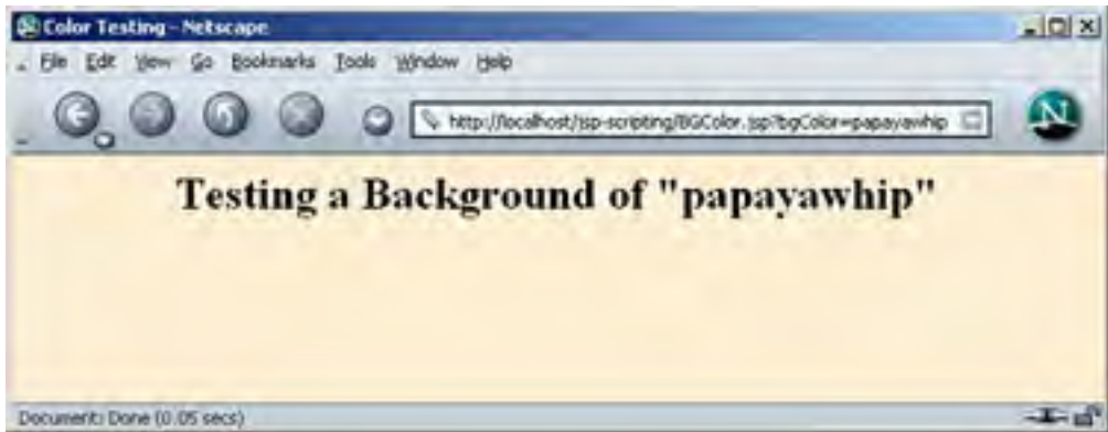
Figure 11-7. Result of BGColor.jsp when accessed with a bgColor parameter having the X11 color name papayawhip .
