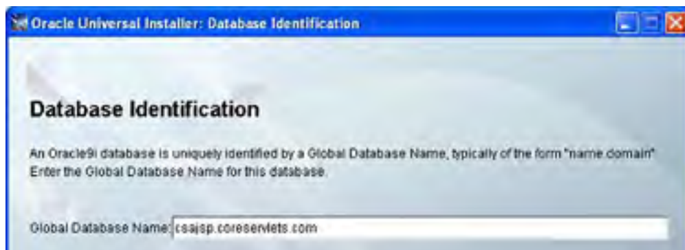
Figure 18-11. Eighth Oracle install window: for specifying the name of the global database and SID.
