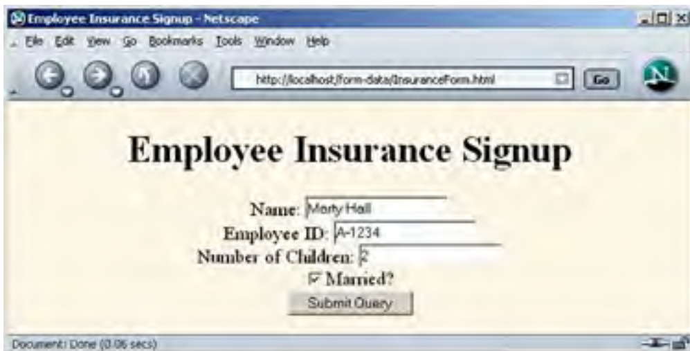
Figure 4-13. Insurance-processing servlet: the gathering of request data is greatly simplified by use of BeanUtilities.populateBean .
