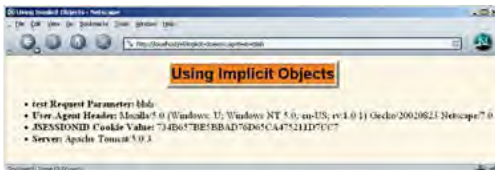
Figure 16-5. A number of scoped variables are defined automatically. These predefined variables are called "implicit objects."
