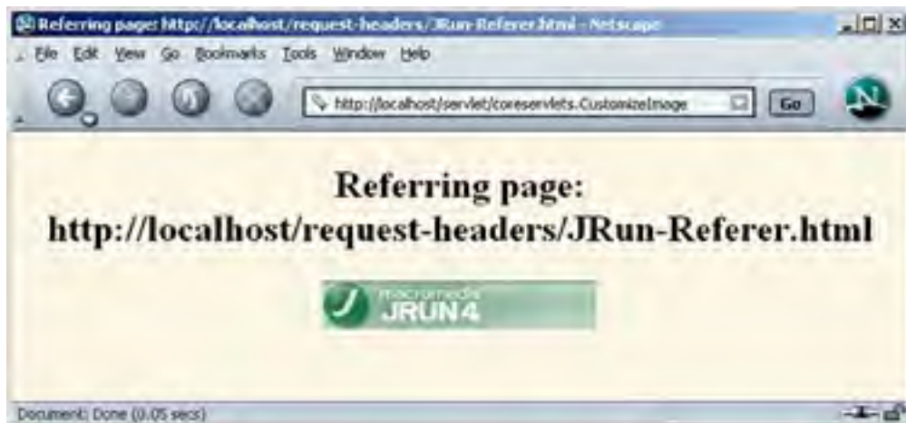
Figure 5-9. The CustomizeImage servlet when the Referer header is missing. When using the Referer header, always handle the case in which the result of getHeader is null .
