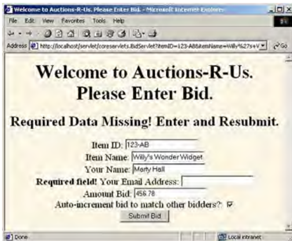
Figure 4-15. Bid servlet with incomplete data. If the user submits a form that is not fully filled in, the bid servlet redisplay the form. The user's previous partial data is maintained, and missing fields are highlighted.
