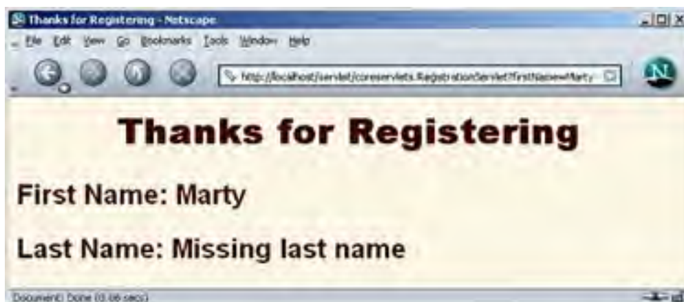
Figure 15-8. Result of RegistrationServlet when one parameter is missing and session data is found.
