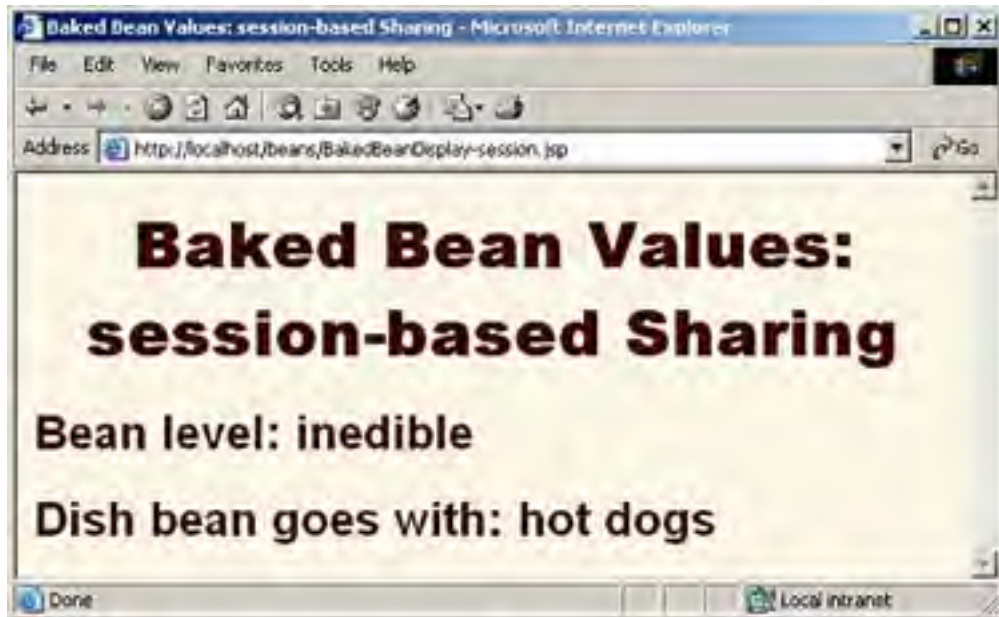
Figure 14-12. Subsequent request to BakedBeanDisplay-session.jsp — BakedBean properties do not persist between requests if the request is from a different client (as here) or is in a different session.
