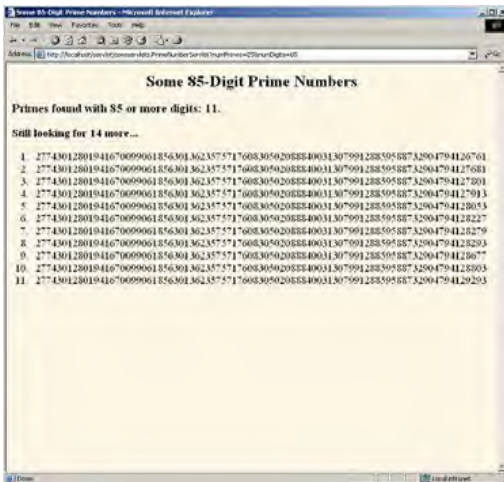
Figure 7-4. Intermediate results of the prime-number-generation servlet. The servlet stores the previous computations and matches the current request with the stored values by comparing the request parameters (the size and number of primes to compute). Other clients that request the same parameters see the same already computed results.
