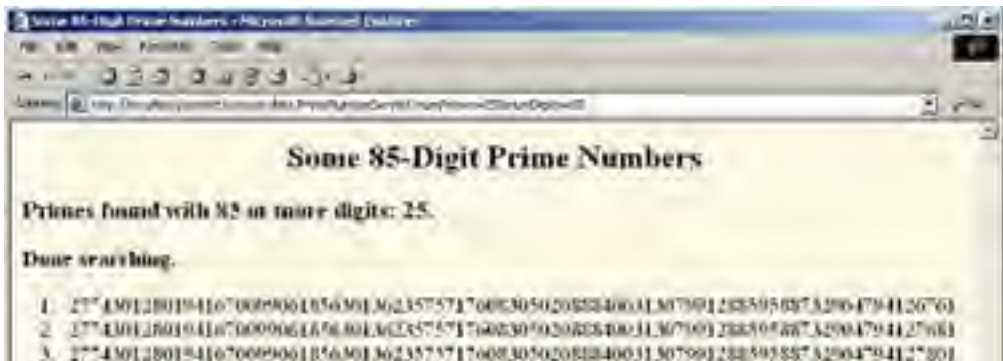
Figure 7-5. Final results of the prime-number-generation servlet. Since the servlet has computed as many primes as the user requested, no Refresh header is sent to the browser and the page is no longer reloaded automatically.
