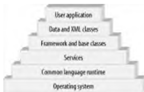
Figure 1-1. .NET Framework architecture
