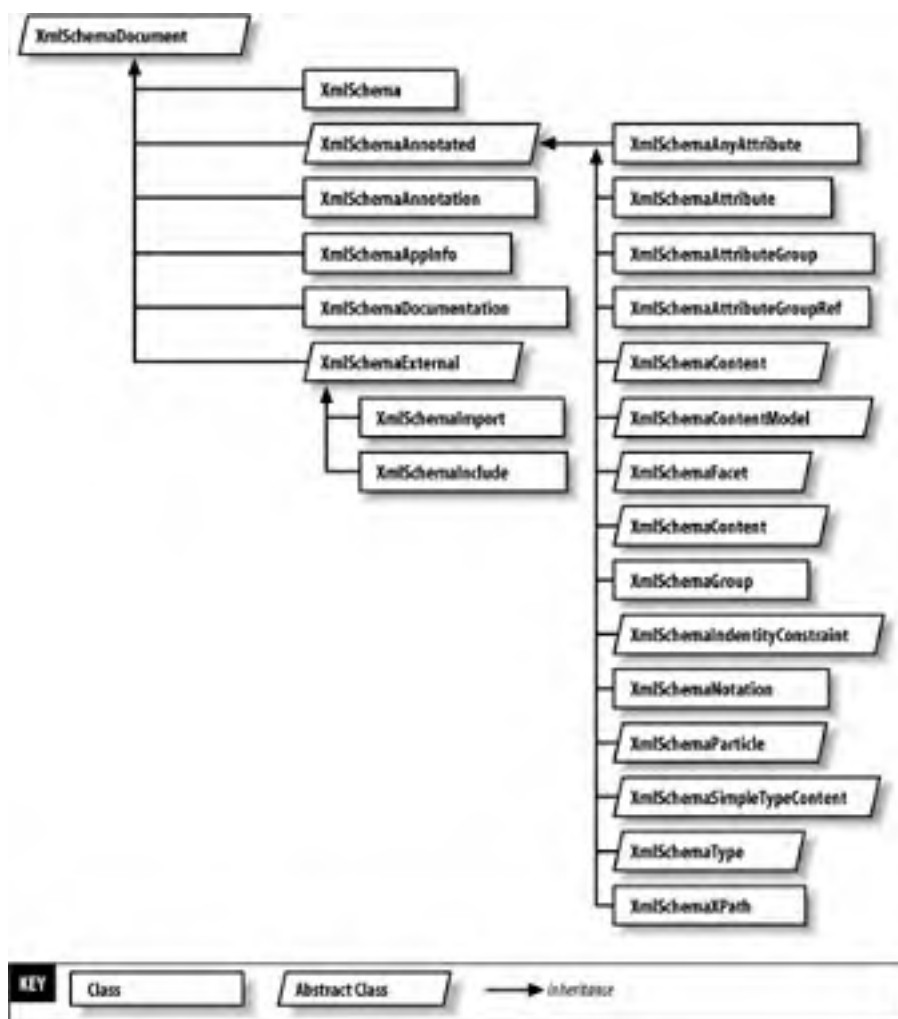
Figure 8-1. XmlSchema type hierarchy
