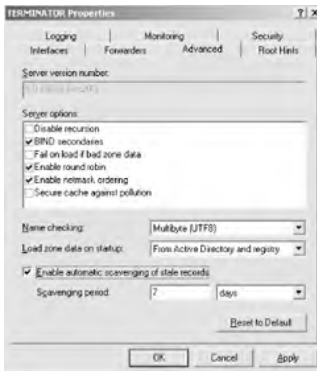
Figure 7-7. Enabling aging and scavenging for an entire server
