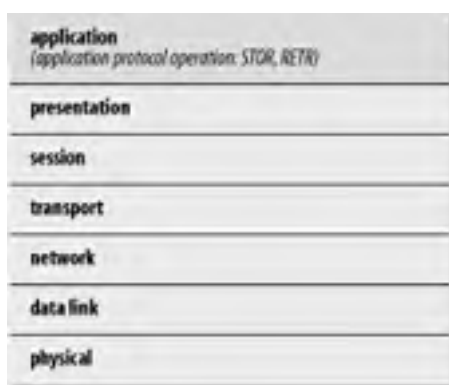
Figure 16-2. Application gateways operate at the application layer of the stack
