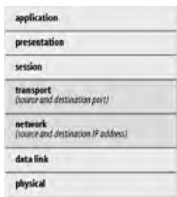
Figure 16-1. Packet filters operate at the network and transport layers of the stack
