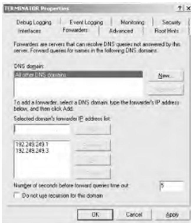
Figure 16-6. Internal name server forwarding configuration
