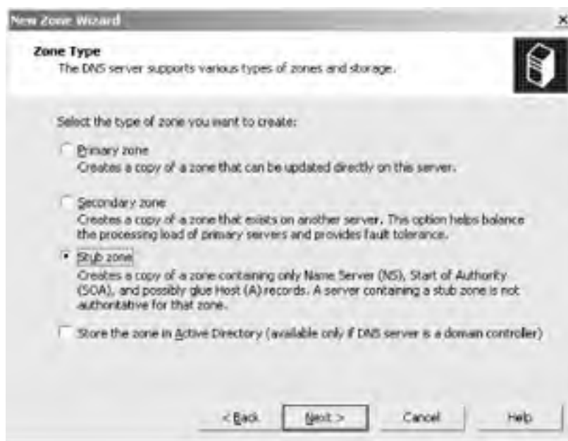
Figure 10-9. Adding a stub zone
