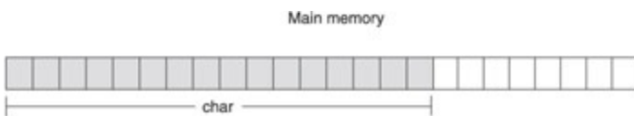
Figure 1-8: A char abstract data type in Java reserves 16 bits of main memory.
