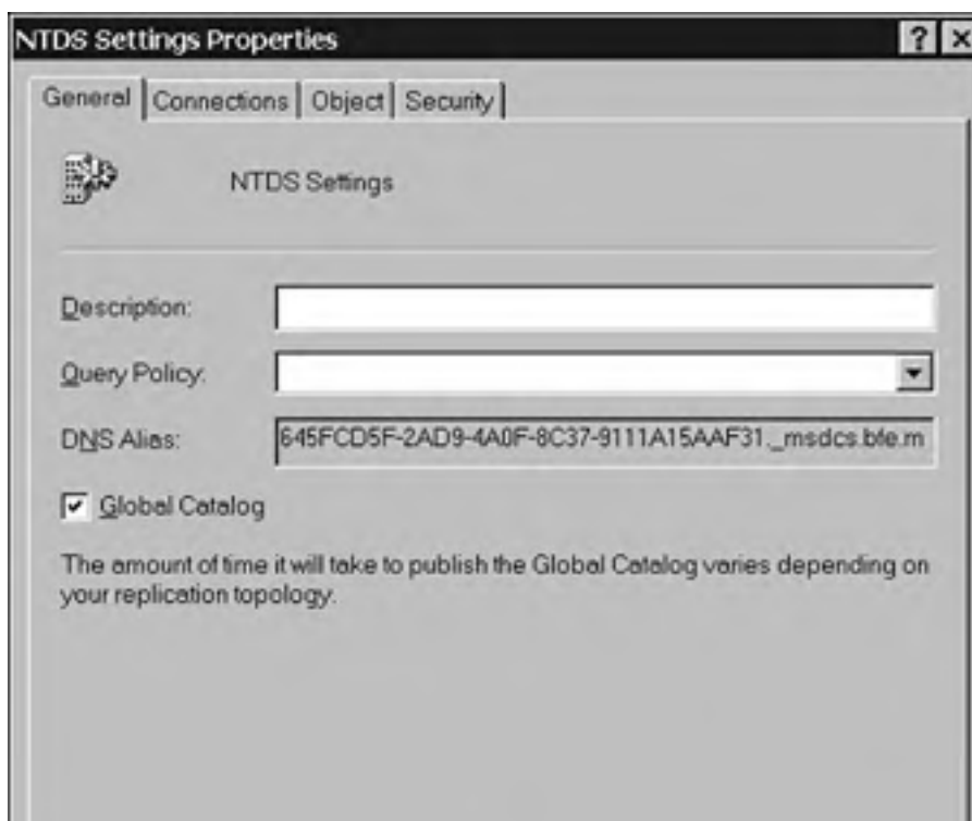
Figure 6.3. You can set any domain controller to be a Global Catalog server.
