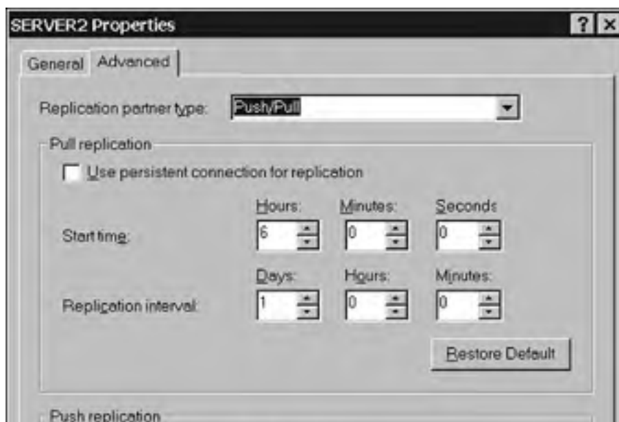
Figure 5.8. You can configure WINS for push/pull replication.
