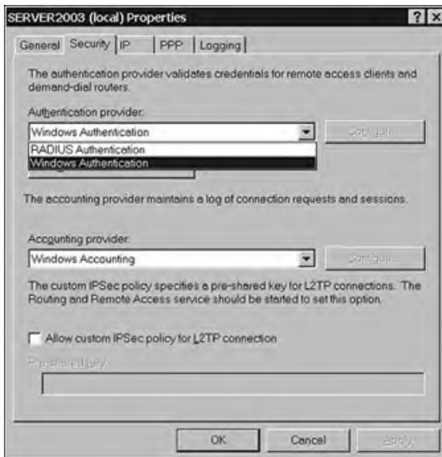
Figure 5.12. You can configure RAS server authentication and logging settings.
