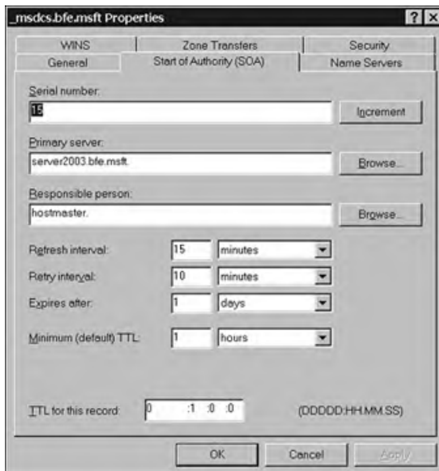
Figure 6.1. Start of authority records control communication between primary and secondary servers.
