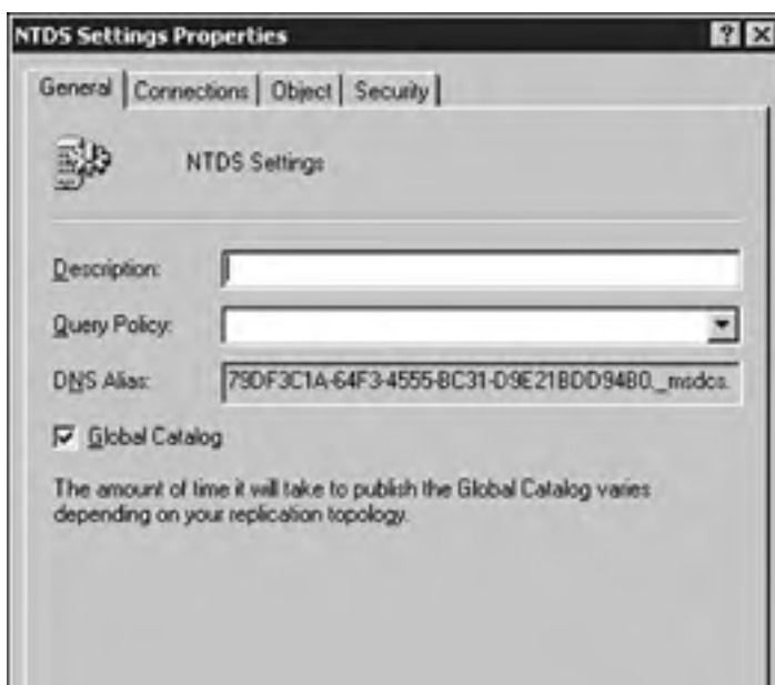
Figure 2.2. Designating a global catalog server.
