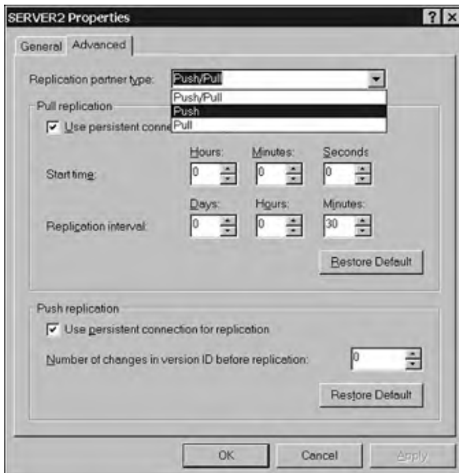
Figure 5.5. You can configure replication for WINS servers.
