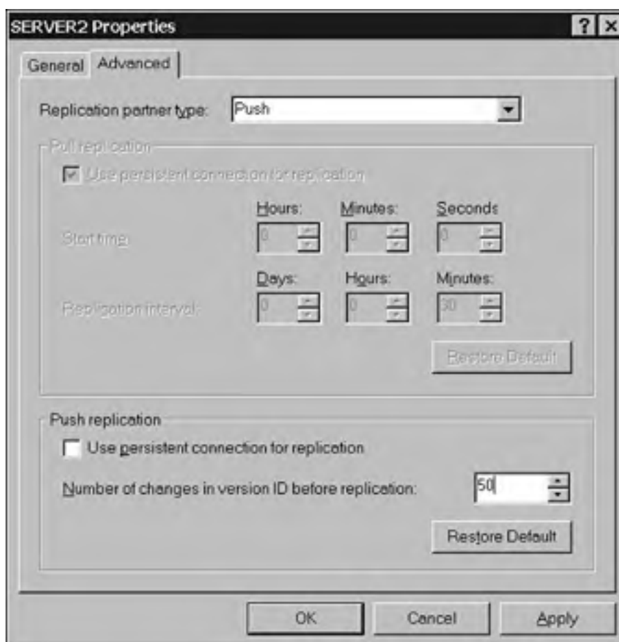
Figure 5.6. You can configure WINS for push replication after 50 changes to the database.
