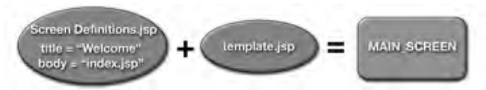
Figure 10.3 Defining a Screen in Terms of a Template and Its Parameters
