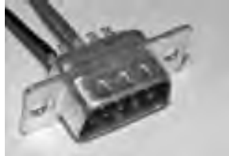
Fig. 13-17. PC asynchronous serial port connectors and pinouts.
