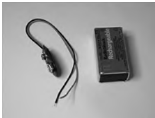
Fig. 3-33. 9 volt battery clip with red (positive) and black (negative) wires attached to it.
