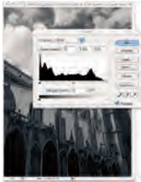
Figure 9-25: The “mountain range” shows the distribution of tonal values in your image.
