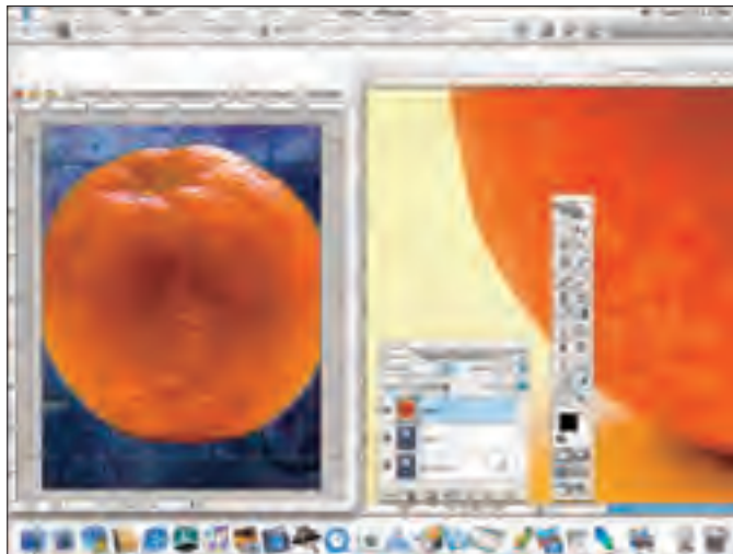
Figure 14-5: Drag anchor points to change the size and shape of the bounding box.
