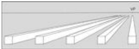
Figure 11-10: Foreshortening creates the illusion that objects look shorter when pointed toward you.
