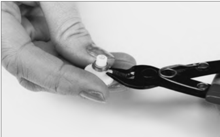
Figure 15-15: Clipping off the ridge on the top of the output gear. Use caution!
