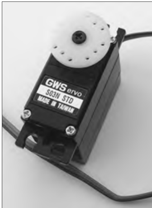
Figure 15-11: A typical standard- size R/C servo motor.
