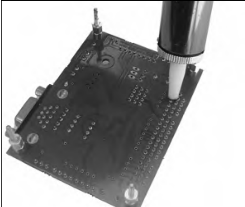
Figure 8-7: Place the nozzle of the desolder pump close to or even touching the solder that you want to remove.
