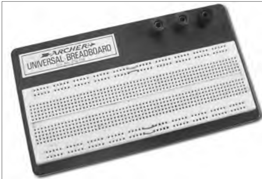
Figure 11-3: For larger circuits, you can use bigger solderless breadboards.
