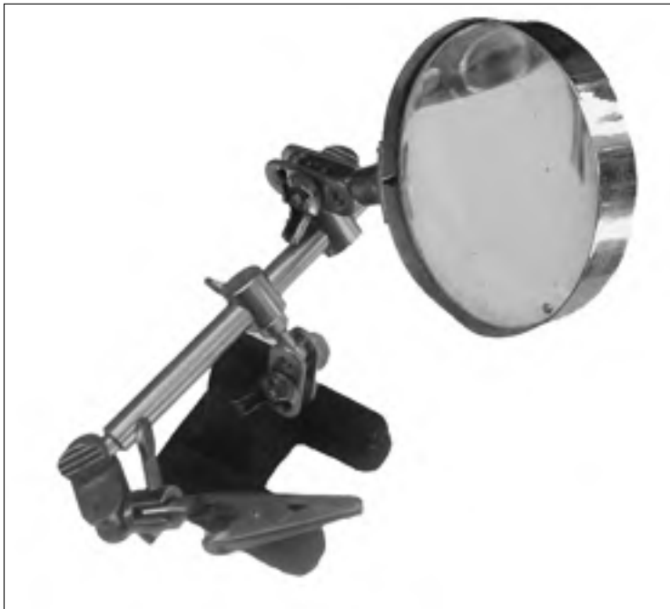
Figure 8-2: A so-called “third hand” clamp helps you hold components while soldering. Get the kind with a built-in magnifier.
