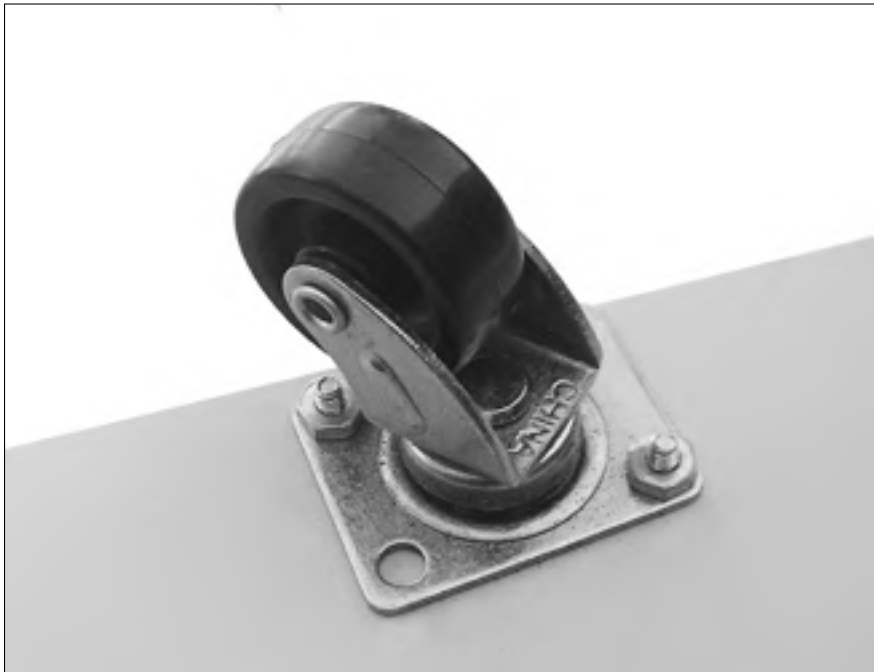
Figure 15-7: Mount the caster to Rover by using 6-32 screws and nuts.
