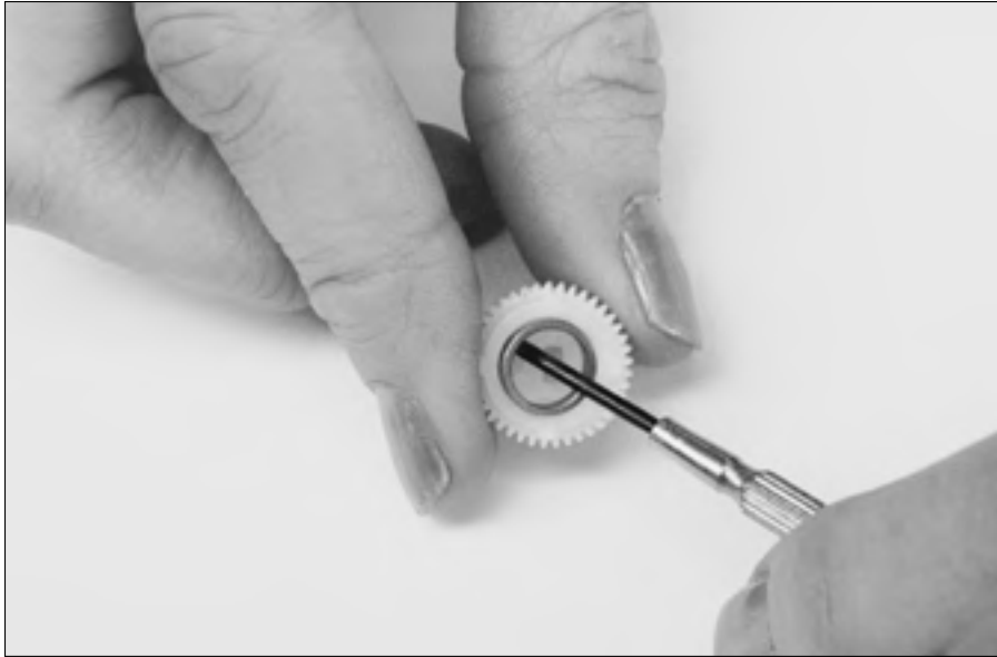
Figure 15-17: Taking out the retainer.
