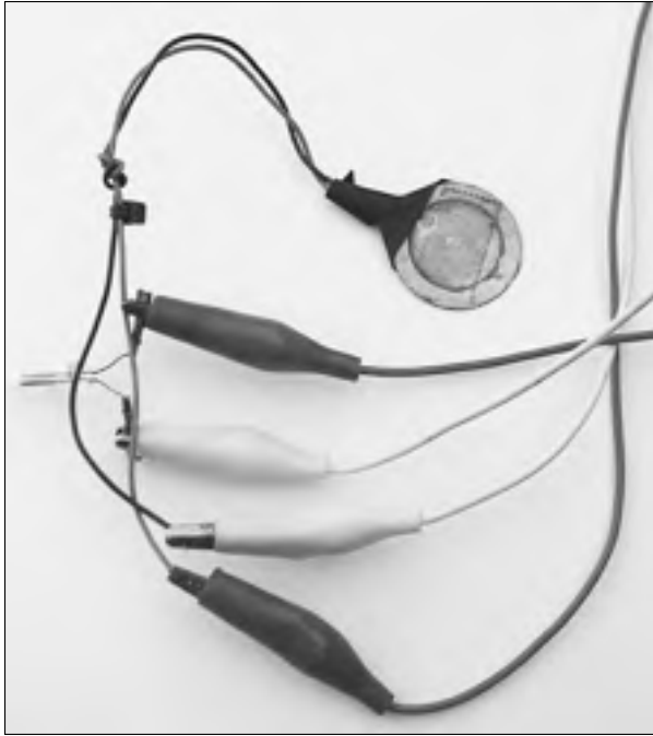
Figure 14-4: Connect the disc and neon lamp, using alligator clips.
