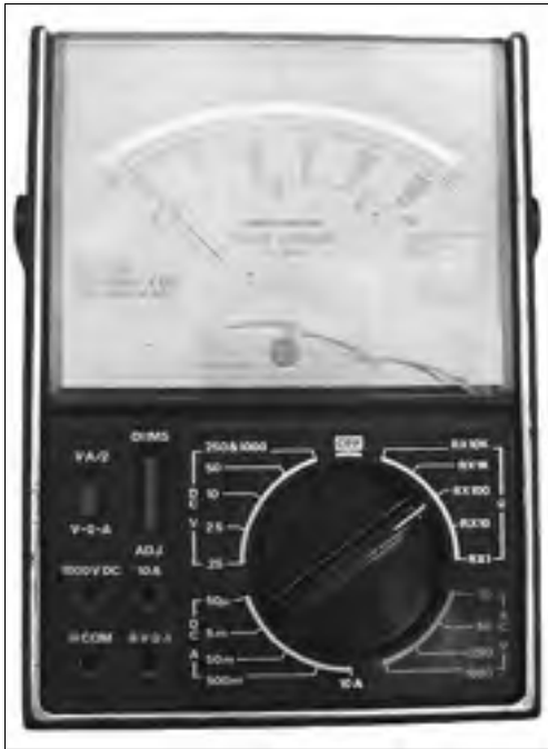
Figure 9-2: An analog multimeter uses a needle to indicate voltage, current, and other values.
