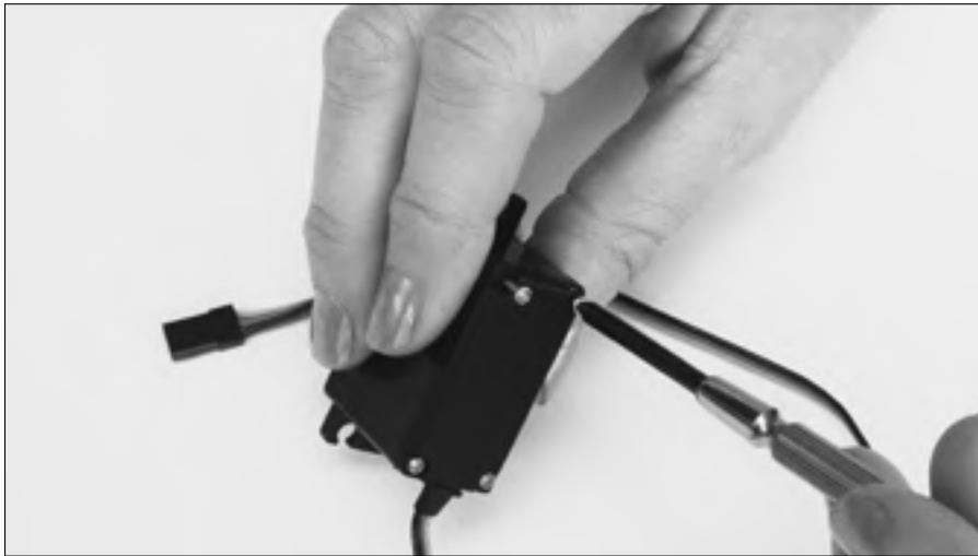
Figure 15-12: Taking the servo apart.
