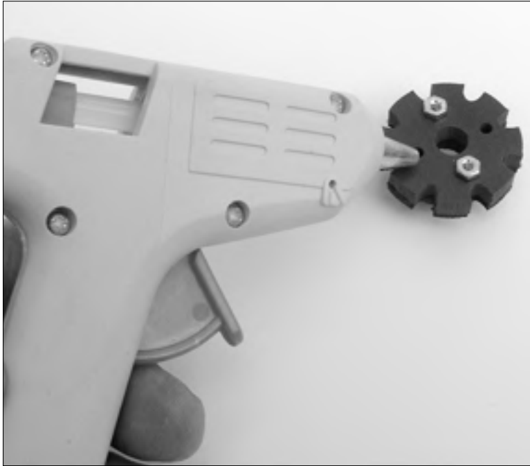
Figure 3-8: A hot-melt glue gun quickly fastens things.
