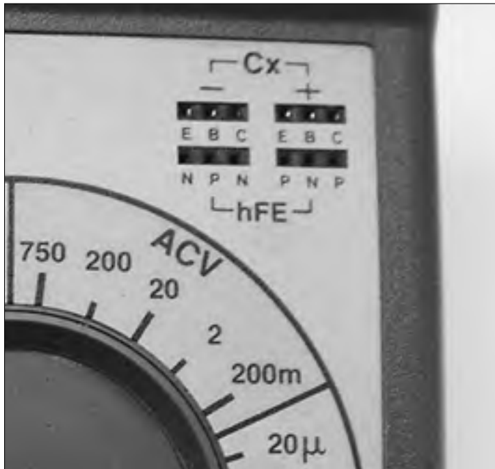
Figure 9-4: Most meters provide additional input sockets for testing capacitors and transistors.
