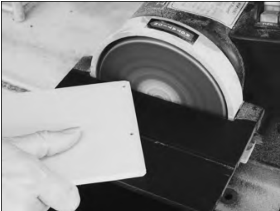
Figure 15-3: Sand down the corners of the robot decks so they are blunted.
