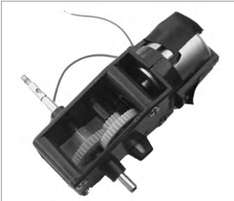
Figure 15-4: A Tamiya gear motor, assembled and ready to go.
