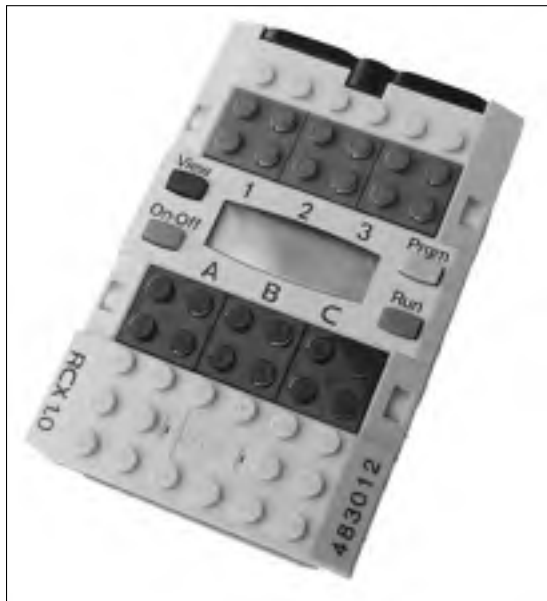
Figure 13-1: The brain of the LEGO Mindstorms robot construction kit contains a micro- controller.
