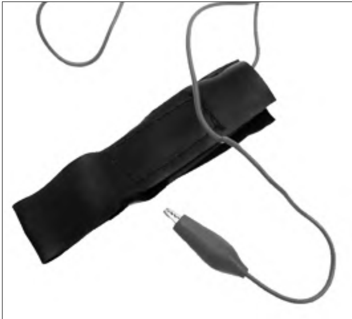
Figure 8-6: An anti-static wrist band helps draw off damage-causing static from your body.
