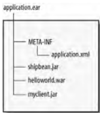
Figure 17-4. Contents of a J2EE .ear file with application component
