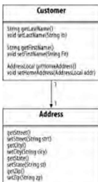
Figure 6-1. Class diagram of Customer and Address EJBs
